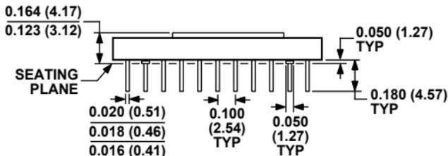
**CONTROLLING DIMENSIONS ARE IN INCHES; MILLIMETER DIMENSIONS (IN PARENTHESES) ARE ROUNDED-OFF INCH EQUIVALENTS FOR REFERENCE ONLY AND ARE NOT APPROPRIATE FOR USE IN DESIGN.**
