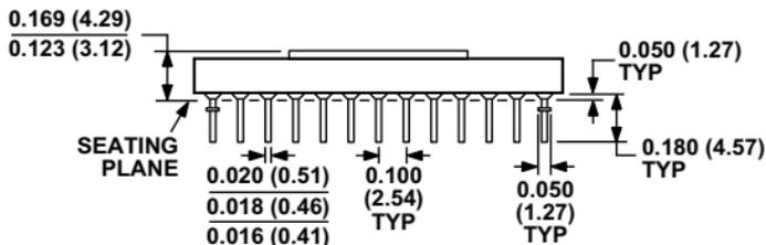
**CONTROLLING DIMENSIONS ARE IN INCHES; MILLIMETER DIMENSIONS (IN PARENTHESES) ARE ROUNDED-OFF INCH EQUIVALENTS FOR REFERENCE ONLY AND ARE NOT APPROPRIATE FOR USE IN DESIGN.**
