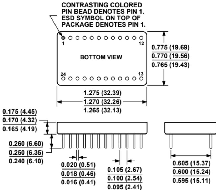
CONTROLLING DIMENSIONS ARE IN INCHES; MILLIMETER DIMENSIONS
