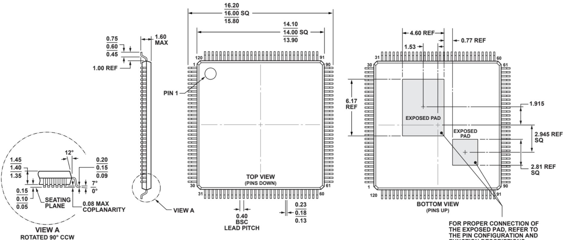
FOR PROPER CONNECTION OF THE EXPOSED PAD, REFER TO THE PIN CONFIGURATION AND FUNCTION DESCRIPTIONS SECTION OF THIS DATA SHEET.
