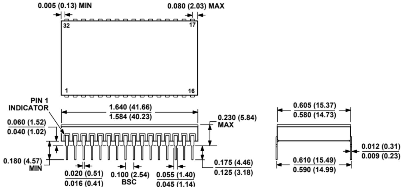
**CONTROLLING DIMENSIONS ARE IN INCHES; MILLIMETER DIMENSIONS
