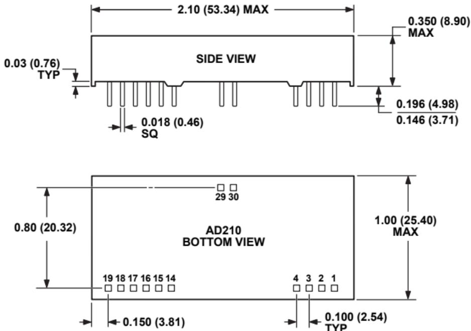
**CONTROLLING DIMENSIONS ARE IN INCHES; MILLIMETER DIMENSIONS (IN PARENTHESES) ARE ROUNDED-OFF INCH EQUIVALENTS FOR REFERENCE ONLY AND ARE NOT APPROPRIATE FOR USE IN DESIGN. CORNER LEADS MAY BE CONFIGURED AS WHOLE OR HALF LEADS.**
