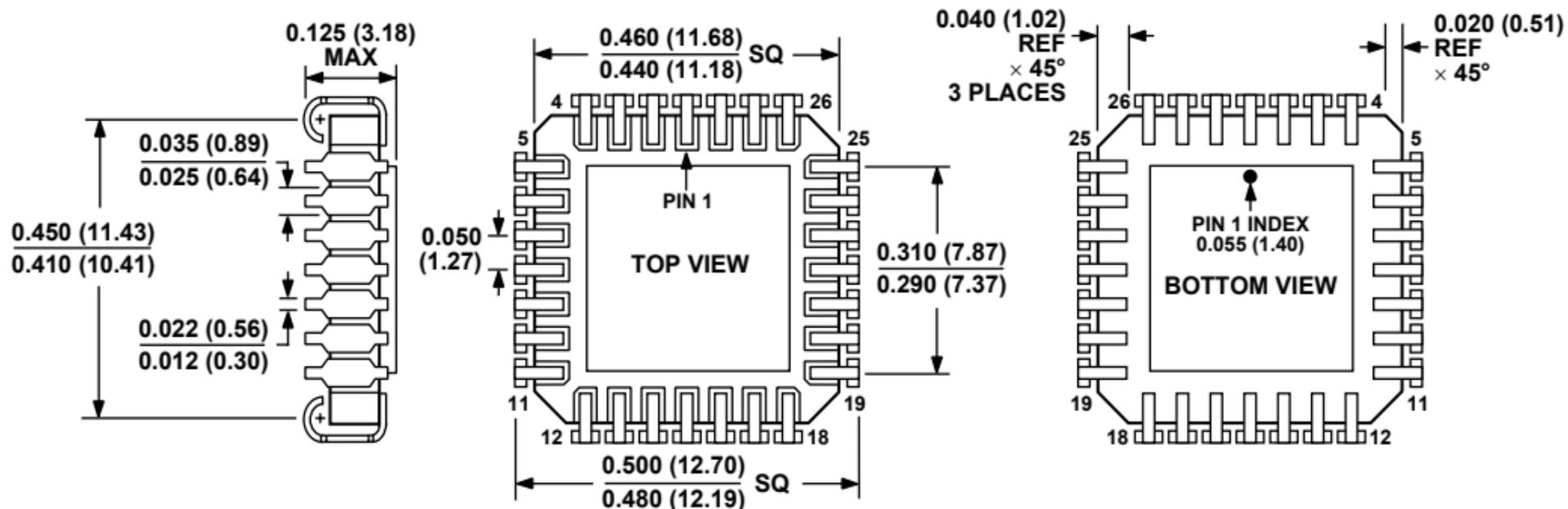
**CONTROLLING DIMENSIONS ARE IN INCHES; MILLIMETERS DIMENSIONS (IN PARENTHESES) ARE ROUNDED-OFF INCH EQUIVALENTS FOR REFERENCE ONLY AND ARE NOT APPROPRIATE FOR USE IN DESIGN.**
