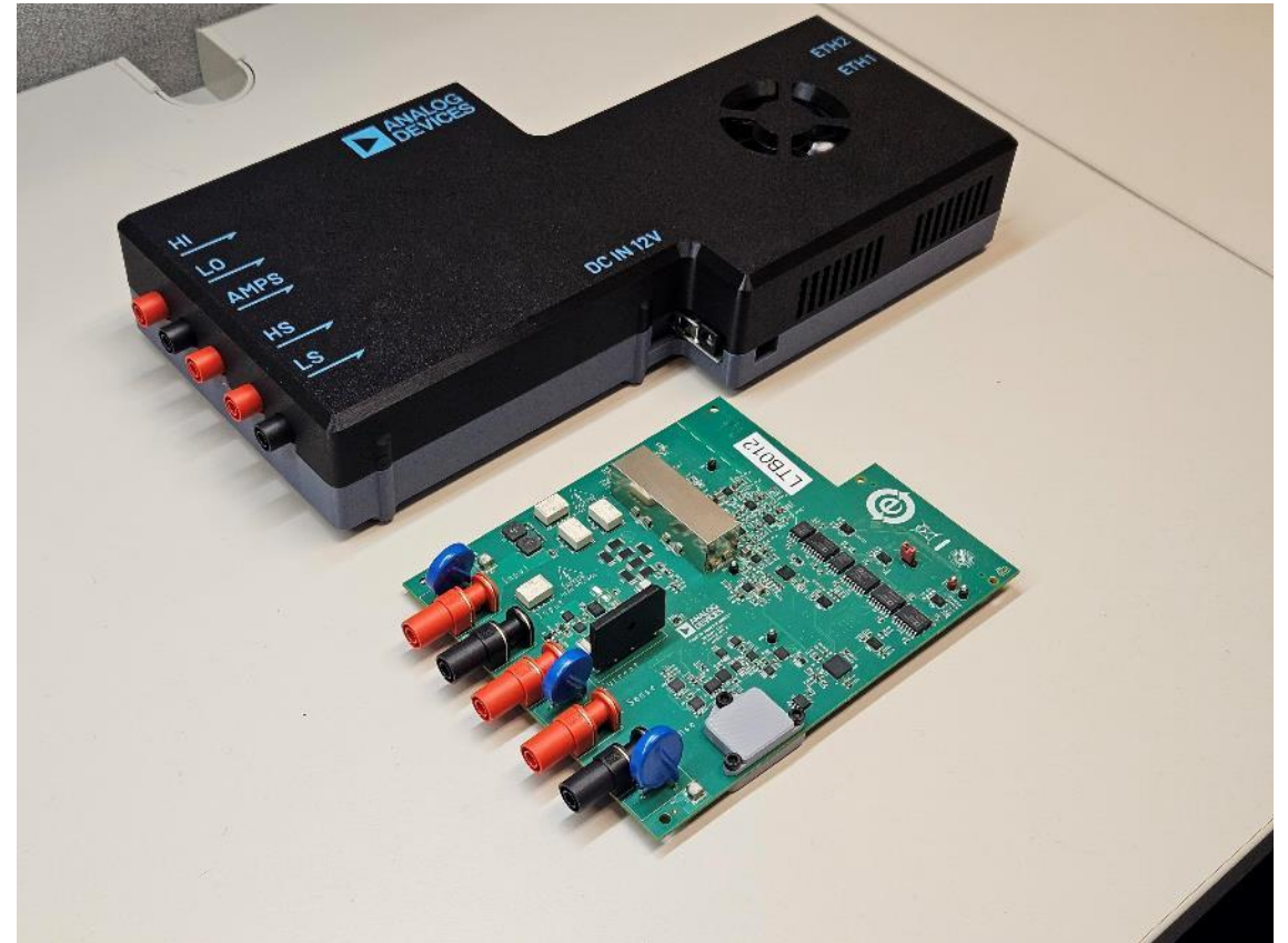
Above: full DMM module Below: DMM analog tile
