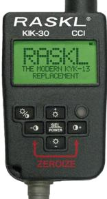
The RASKL® device is a ruggedized, portable handheld device for securely receiving, storing, and transferring data between compatible cryptographic and communications equipment. The ReAlly Simple Key Loader (RASKL) is the first NSA Certified KYK-13 replacement.
