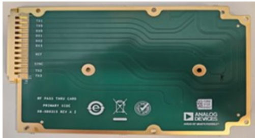
Passthru Tuner, 1st and/or 2nd Nyquist for Direct-Sampling
