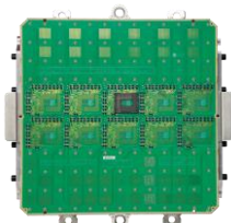
Example ATE load board (high-speed loopback + DC test)
