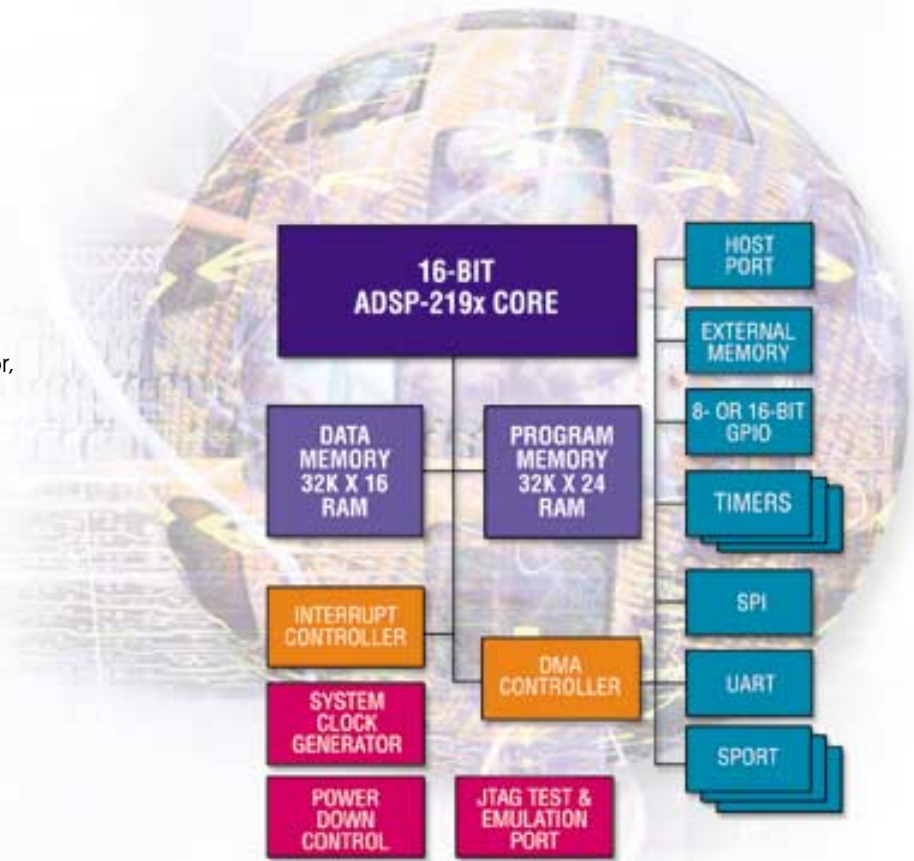
ADSP-2191 FUNCTIONAL BLOCK DIAGRAM
