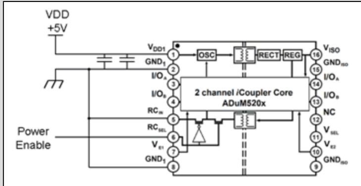
Figure 2 - Power Shut Down
