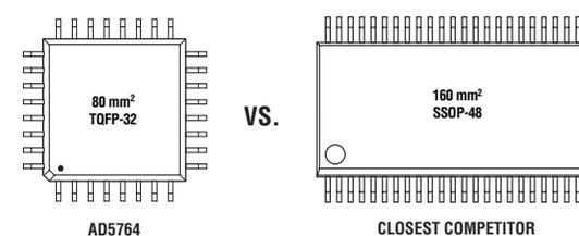
Figure 2. The quad 16-bit DAC (AD5764) cuts board space in half, and has triple the accuracy of the closest competitor.
