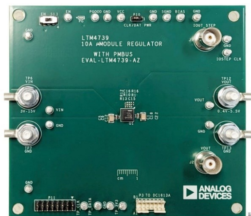
Figure 1. EVAL-LTM4739-AZ Evaluation Board (Part Marking is either ink Mark or Laser Mark)
