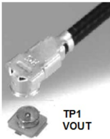
Figure 3. Technique for Measuring Output Ripple and Step Response with a Low Inductance Connector (Not Supplied)
