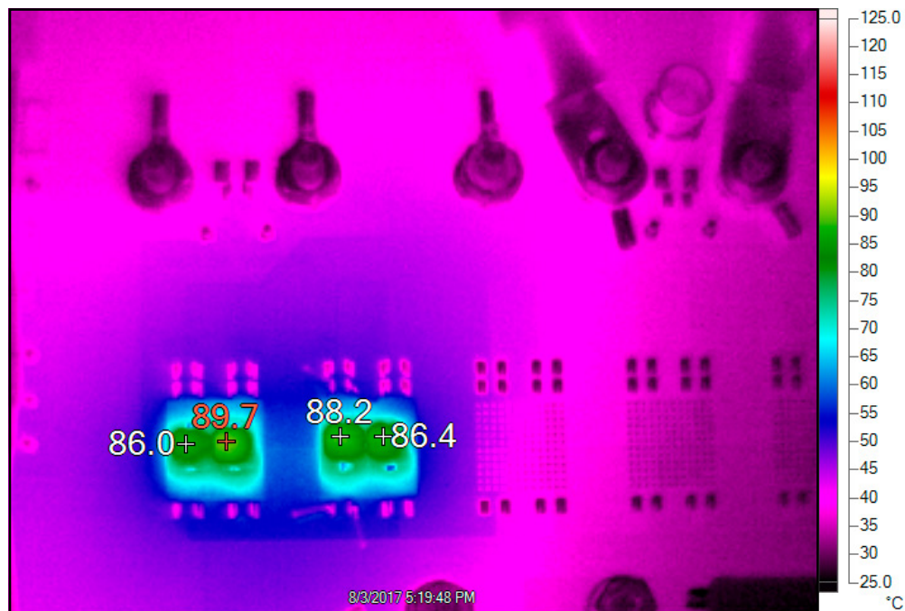
Figure 8. Thermal @ V_{IN} = 12V , V_{OUT} = 1.0V , I_{OUT} = 78A , T_A = 25^{\circ}C , No Airflow
