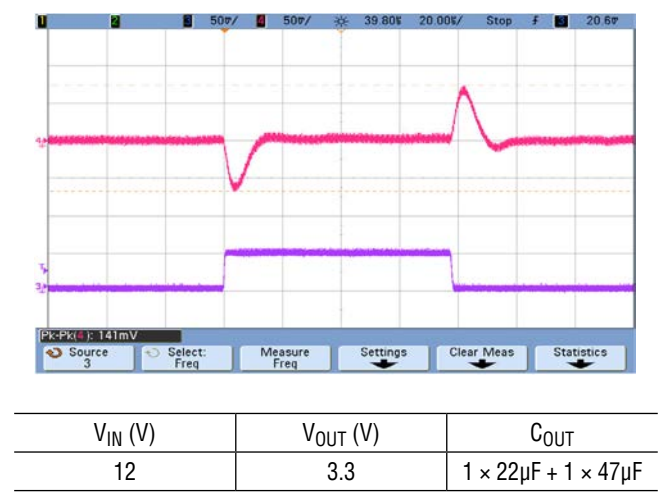
Figure 4. Measured Load Transient Response (1A to 2A Load Step)
