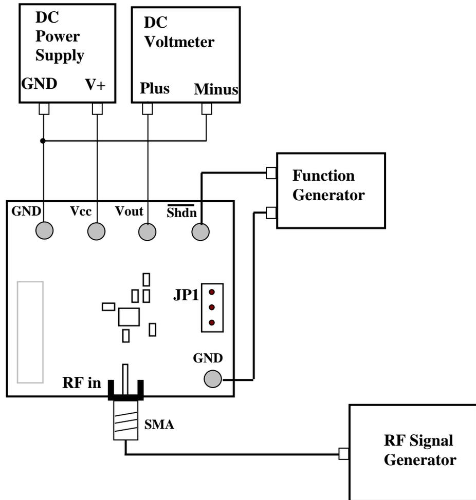
**DC539B Demo Board Connection Diagram**
