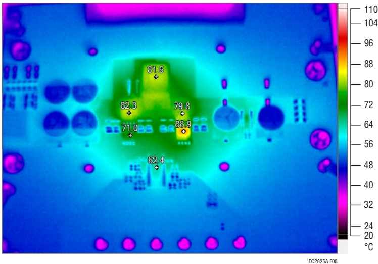
Figure 8. Temperature at Worst-Case ( V_{IN} = 9.25V , V_{OUT} = 12V , I_{OUT} = 10A , SSFM ON)
