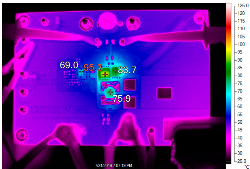
Figure 7. Thermal performance V_{IN} = 24V , V_{OUT} = 3.3V , I_{OUT} = 10A T_A = 23^\circ C , No Airflow
