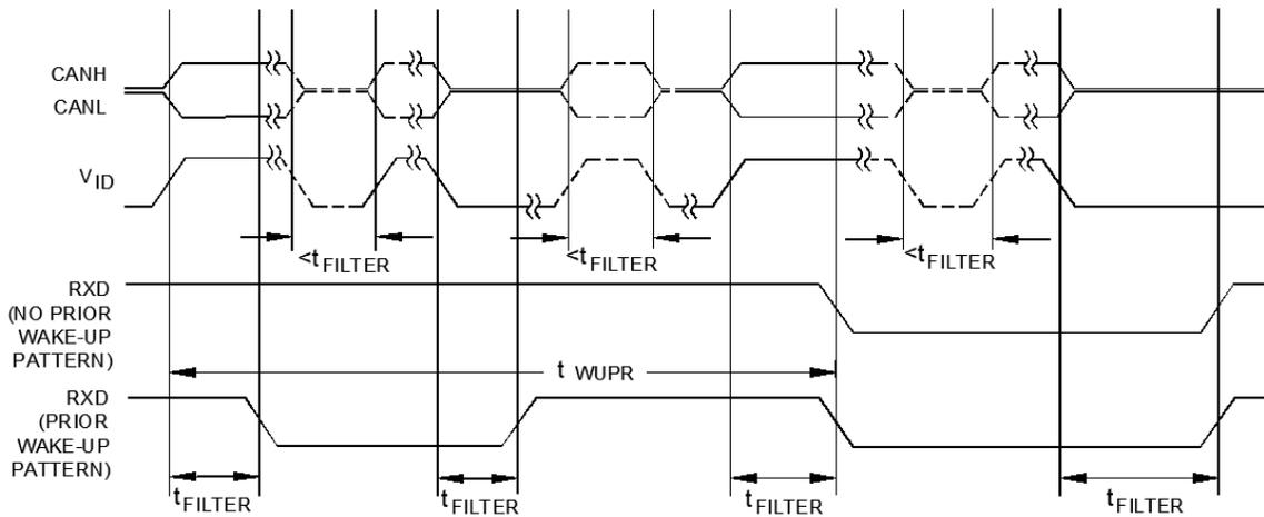
FIGURE 9. Wake up pattern detection and filtered RXD in standby mode timing diagram.
