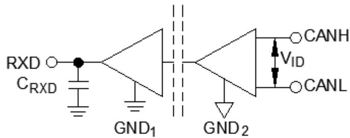
FIGURE 5. Receiver voltage measurement.
