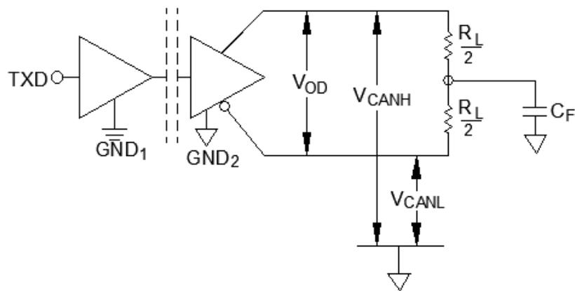
FIGURE 4. Driver voltage measurement.
