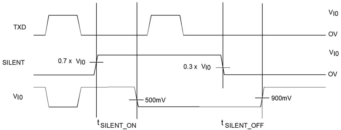
FIGURE 10. Silent mode timing diagram.
