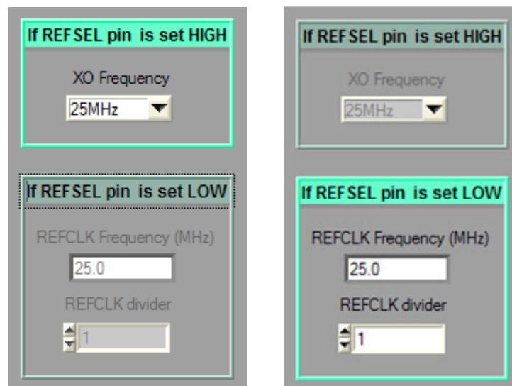
Figure 7. The two states of the input frequency configuration
