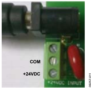
Figure 11. Power Connections
