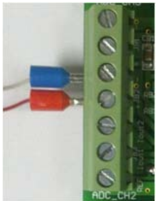
Figure 7. Thermocouple Connector
