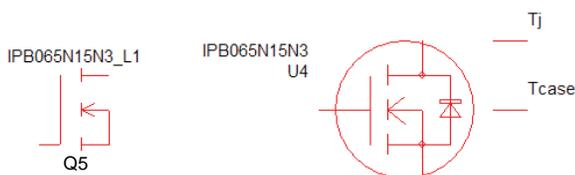
Figure 8. 3-Pin and 5-Pin N-Channel FET Symbols
