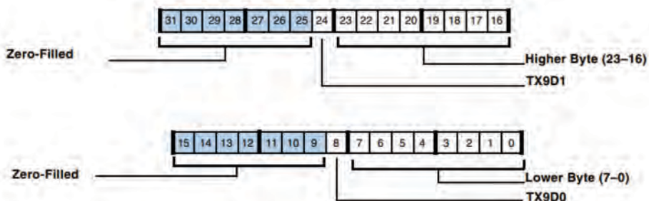
Figure 16-3. UART0 Transmit Holding Register (Packing Enabled)
