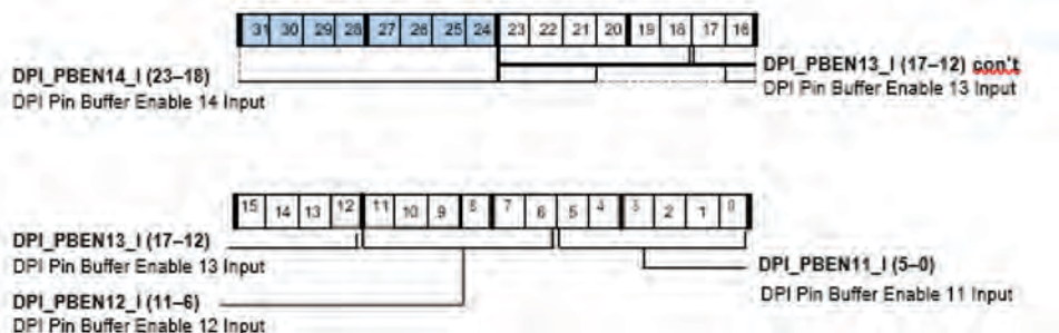
Figure A-53. SRU2_PBEN2 Register
