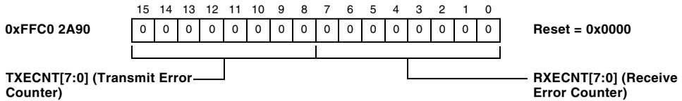
Figure 19-61. Error Counter Register
