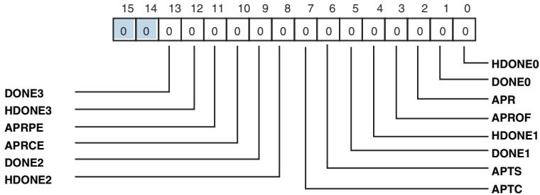
Figure 21-9. MXVR Interrupt Status Register\_1 (MXVR\_INT\_STAT\_1)
