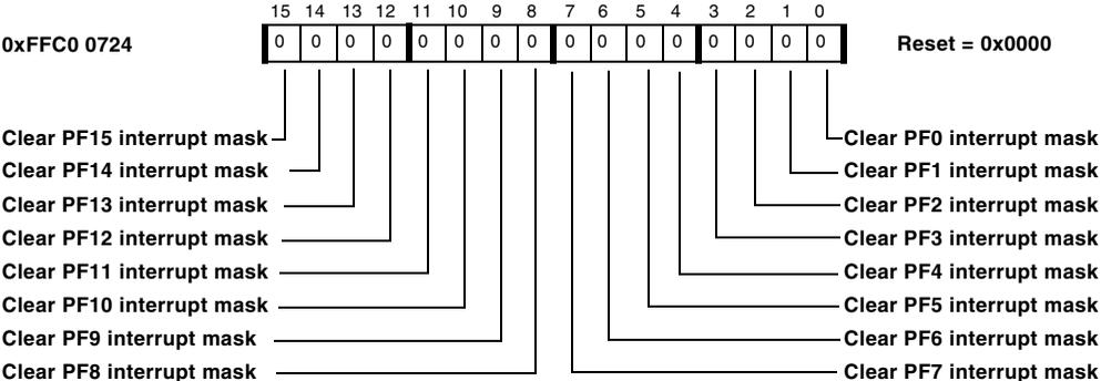
Figure 14-13. Flag Mask Interrupt B Clear Register
