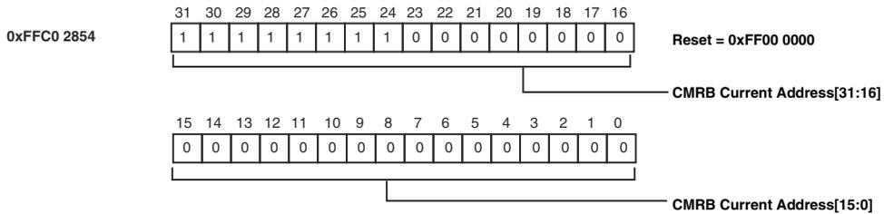
Figure 21-33. MXVR Control Message Receive Buffer Current Address Register (MXVR\_CMRB\_CURR\_ADDR)
