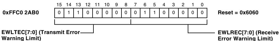
Figure 19-63. Error Counter Warning Level Register
