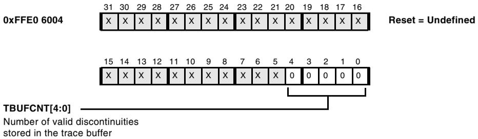
Figure 23-10. Trace Buffer Status Register
