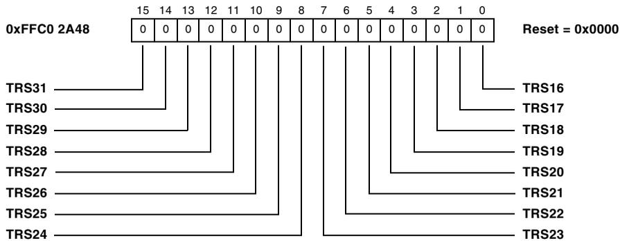
Figure 19-42. Transmission Request Set Register 2
