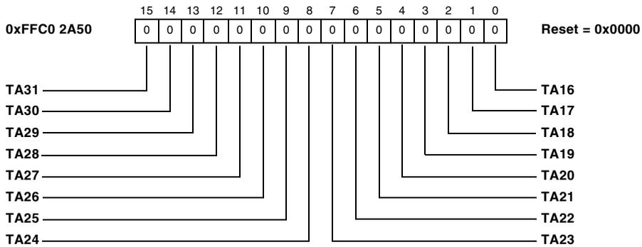
Figure 19-48. Transmission Acknowledge Register 2
