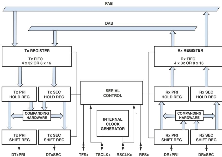
NOTE 1: ALL WIDE ARROW DATA PATHS ARE 16 OR 32 BITS WIDE, DEPENDING ON SLEN. FOR SLEN = 2 TO 15, A 16-BIT DATA PATH WITH 8-DEEP FIFO IS USED. FOR SLEN = 16 TO 31, A 32-BIT DATA PATH WITH 4-DEEP FIFO IS USED.
