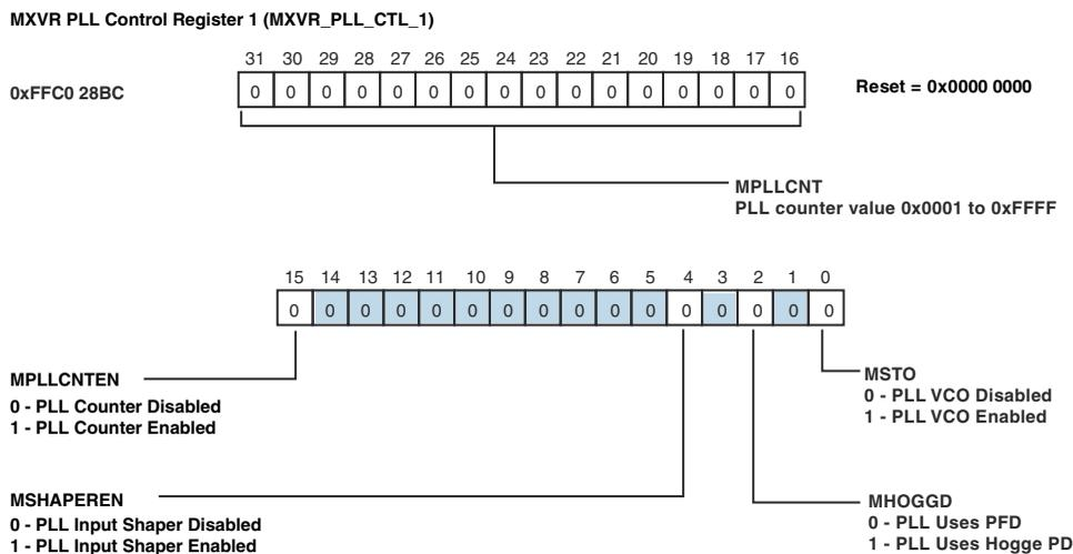
Figure 21-4. MXVR PLL Control Register 1 (MXVR\_PLL\_CTL\_1)
