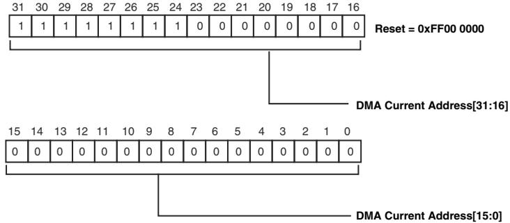
Figure 21-23. MXVR DMA Channel x Current Address Register (MXVR\_DMAx\_CURR\_ADDR)
