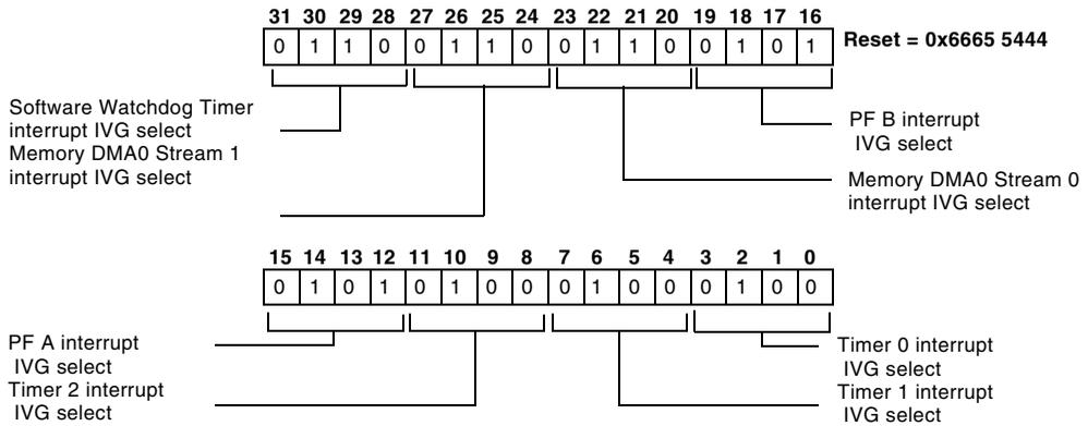
Figure 4-14. System Interrupt Assignment Register 2 (SIC\_IAR2)
