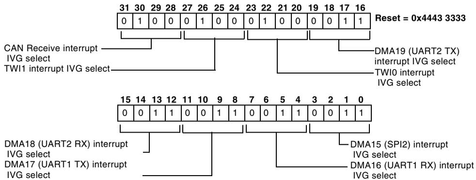
Figure 4-17. System Interrupt Assignment Register 5 (SIC\_IAR5)
