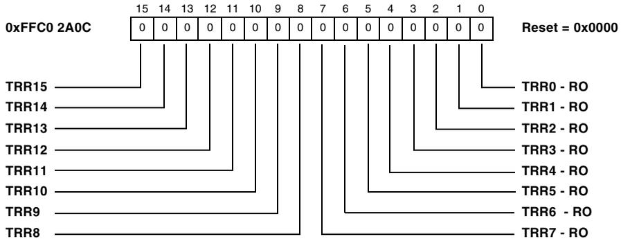
Figure 19-43. Transmission Request Reset Register 1
