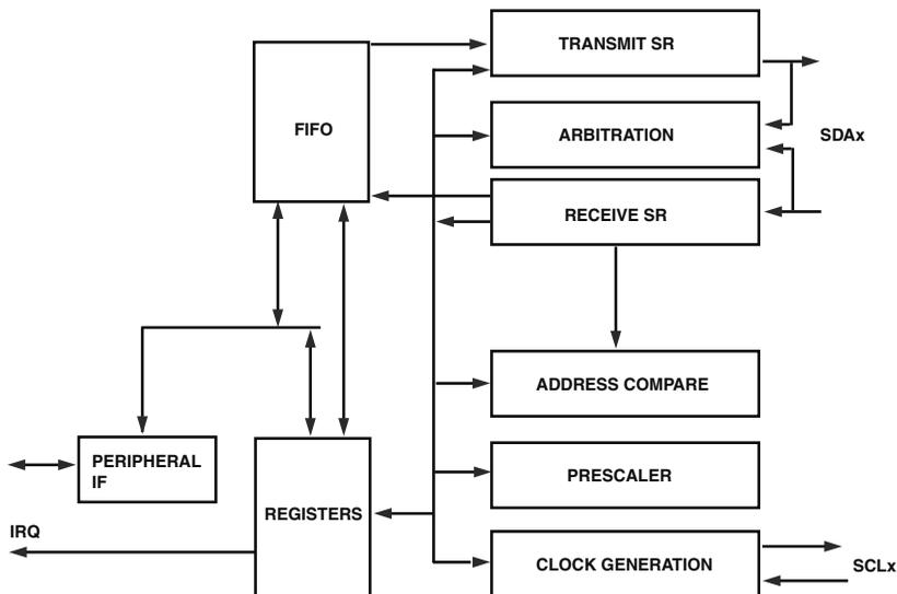
Figure 20-1. TWI Block Diagram
