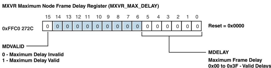
Figure 21-15. MXVR Maximum Node Frame Delay Register (MXVR\_MAX\_DELAY)
