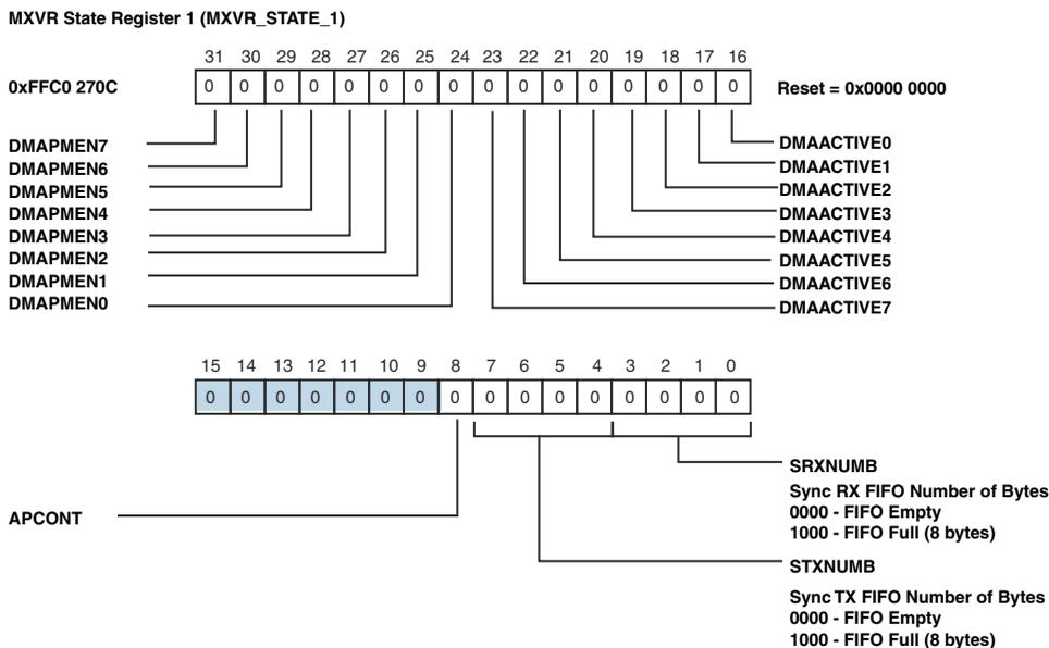
Figure 21-7. MXVR State Register (MXVR\_STATE\_1)
