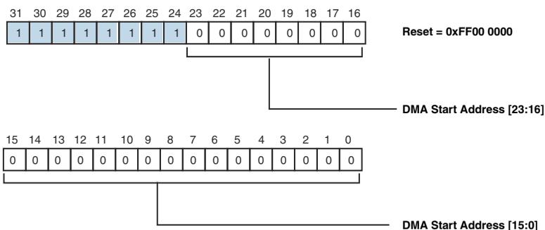
Figure 21-22. MXVR DMA Channel x Start Address Registers
