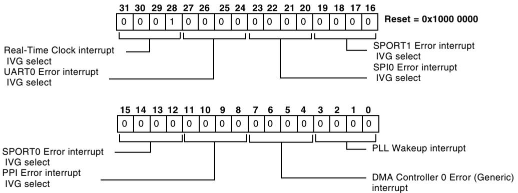
Figure 4-12. System Interrupt Assignment Register 0 (SIC\_IAR0)
