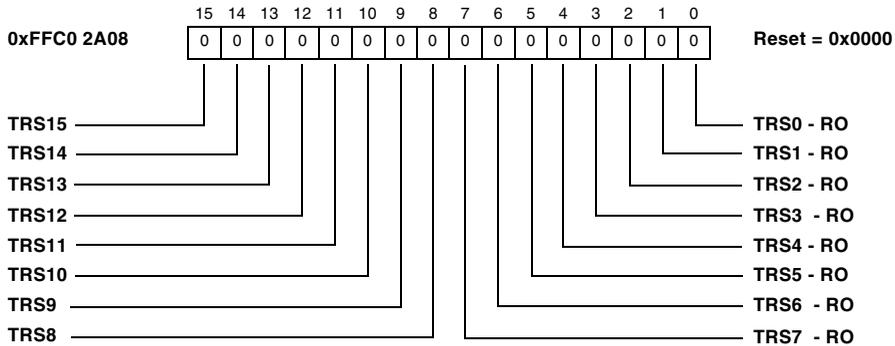
Figure 19-41. Transmission Request Set Register 1
