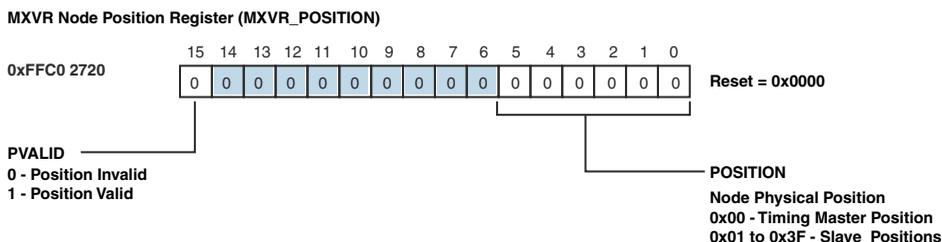
Figure 21-12. MXVR Node Position Register (MXVR\_POSITION)
