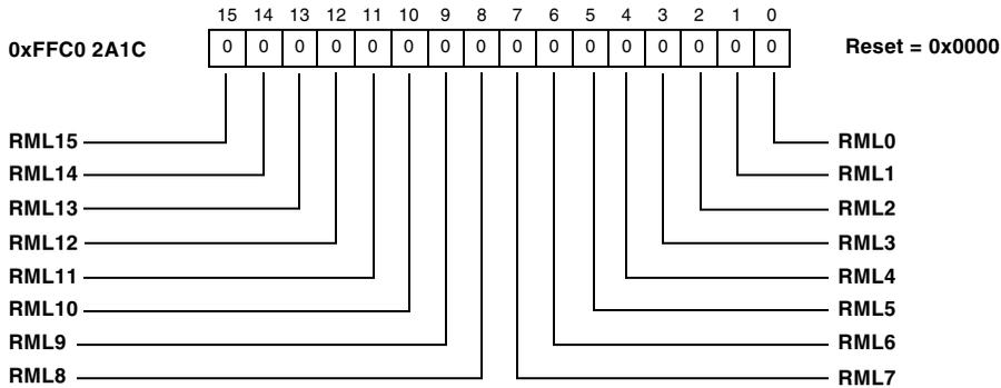
Figure 19-37. Receive Message Lost Register 1
