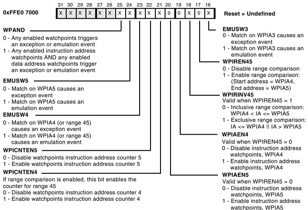
Figure 23-3. Instruction Watchpoint Address Control Register (WPIACTL)[31:16]
