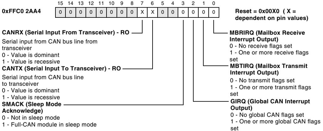
Figure 19-17. CAN Interrupt Register
