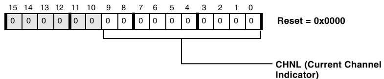
Figure 12-26. SPORT<sub>x</sub> Current Channel Register
