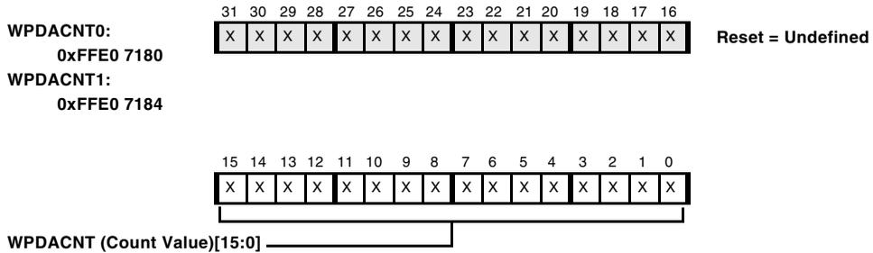
Figure 23-6. Data Watchpoint Address Count Value Registers
