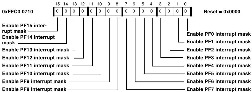
Figure 14-7. Flag Mask Interrupt A Data Register
