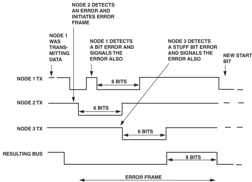
Figure 19-11. CAN Error Scenario Example
