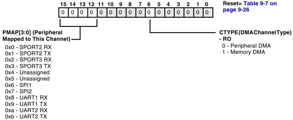
Figure 9-13. DMA Controller 1 Peripheral Map Register
