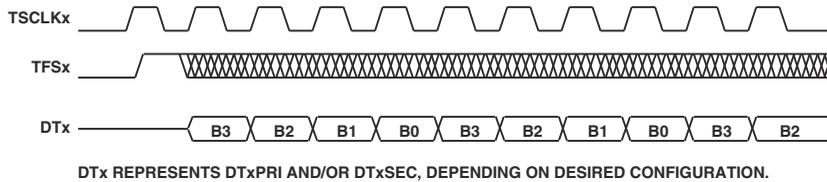
Figure 12-40. SPORT Transmit, Unframed Mode, Normal Framing
