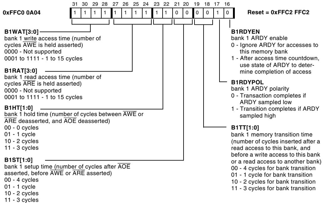
Figure 18-4. Asynchronous Memory Bank Control 0 Register (Bits 31–16)
