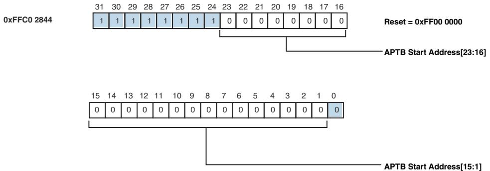
Figure 21-29. MXVR Asynchronous Packet Transmit Buffer Start Address Register (MXVR\_APTB\_START\_ADDR)
