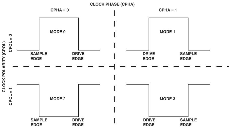
Figure 10-11. SPI Modes of Operation
