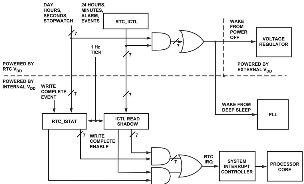
Figure 17-3. RTC Interrupt Structure
