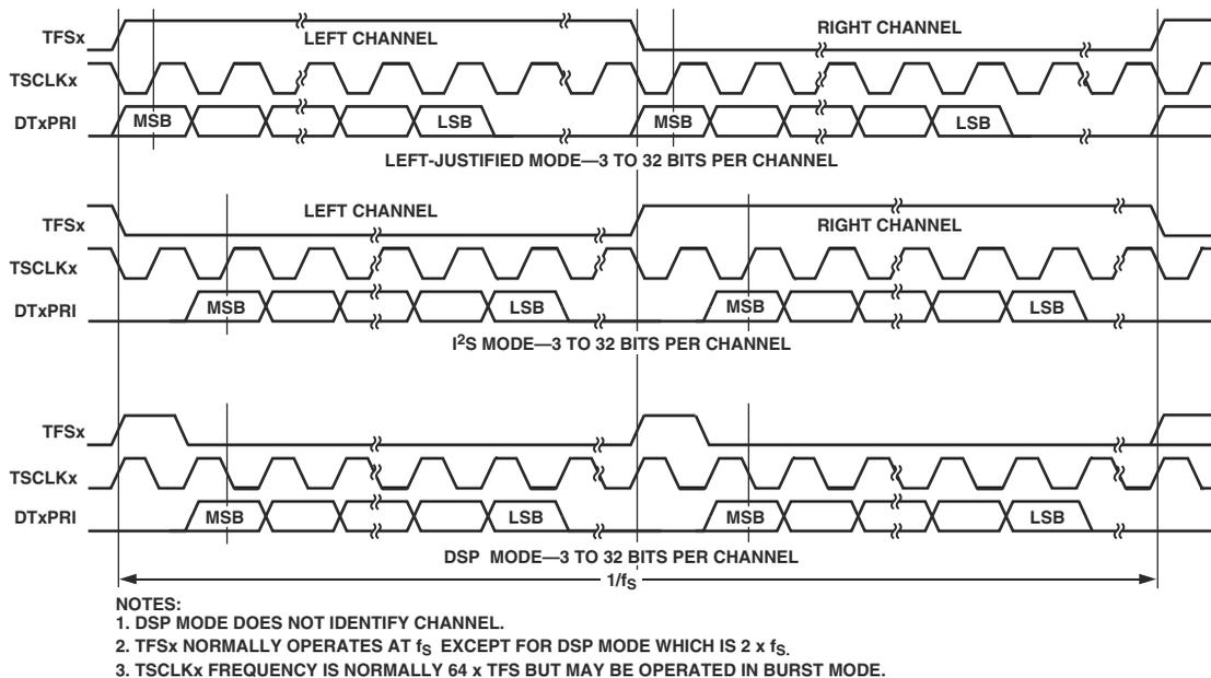
Figure 12-20. SPORT Stereo Serial Modes, Transmit
