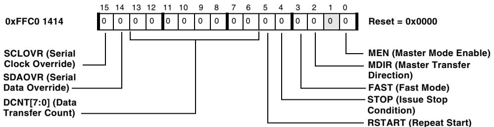
Figure 20-7. TWI Master Mode Control Registers
