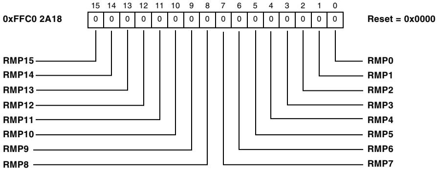
Figure 19-35. Receive Message Pending Register 1
