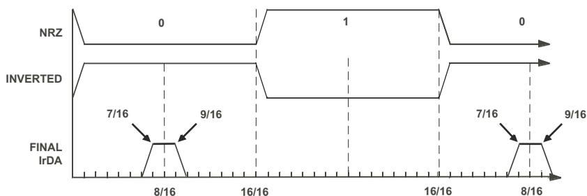
Figure 13-12. IrDA Transmit Pulse
