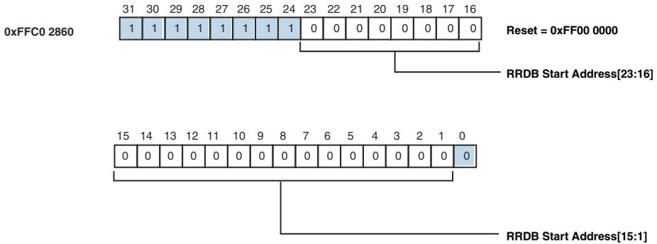
Figure 21-36. MXVR Remote Read Buffer Start Address Register (MXVR\_RRDB\_START\_ADDR)
