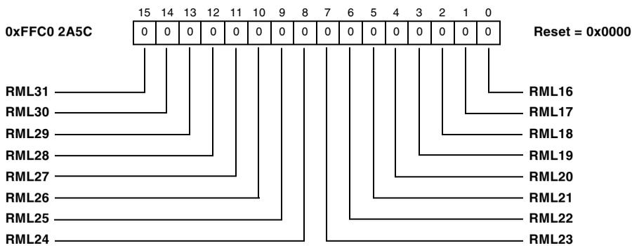
Figure 19-38. Receive Message Lost Register 2
