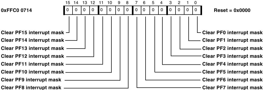
Figure 14-9. Flag Mask Interrupt A Clear Register
