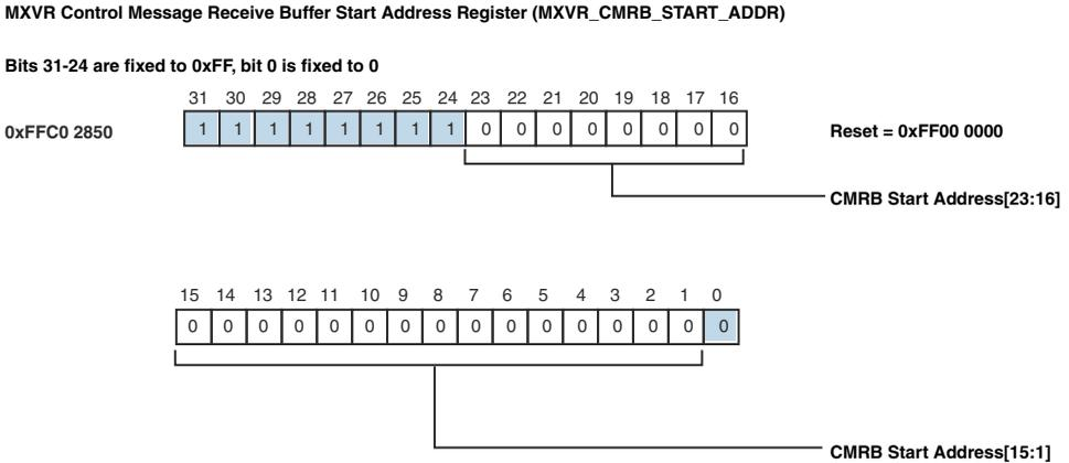
Figure 21-32. MXVR Control Message Receive Buffer Start Address Register (MXVR\_CMRB\_START\_ADDR)
