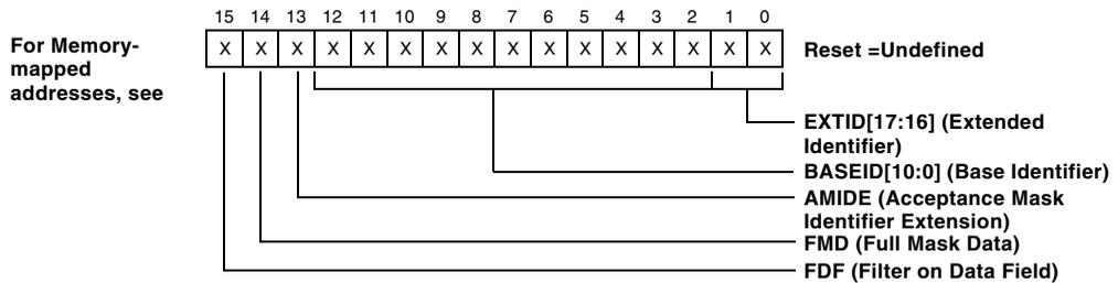
Figure 19-21. Acceptance Mask Register (H)
