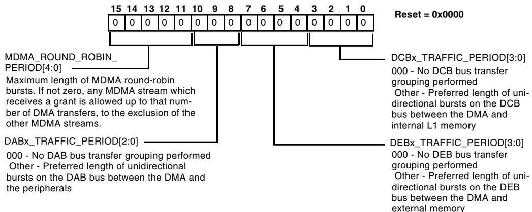
Figure 9-18. DMA Traffic Control Counter Period Register
