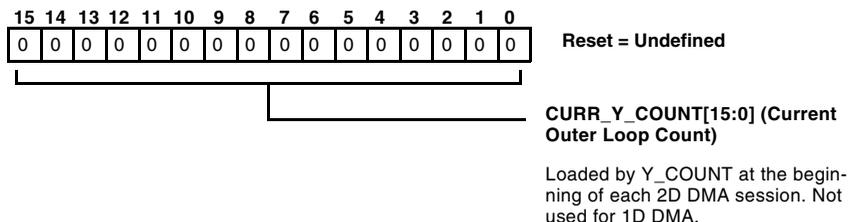
Figure 9-11. Current Outer Loop Count Register
