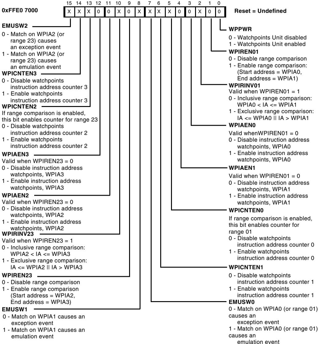
Figure 23-4. Instruction Watchpoint Address Control Register (WPIACTL)[15:0]
