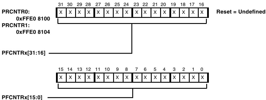
Figure 23-12. Performance Monitor Counter Registers
