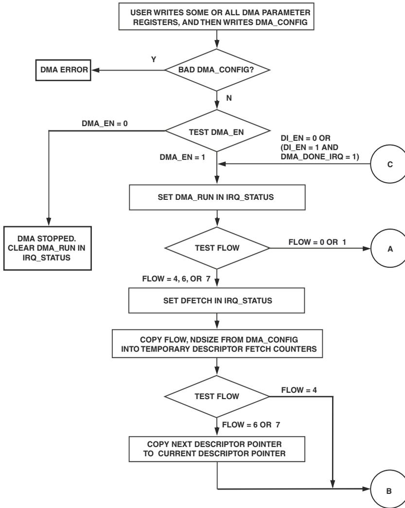
Figure 9-16. DMA Flow, from DMA Controller point of view (1 of 2)
