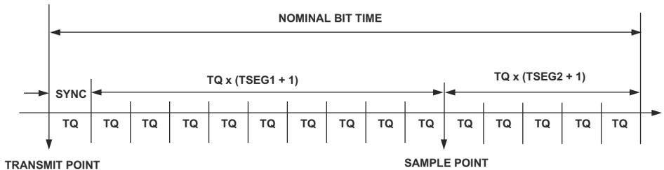
Figure 19-7. Three Phases of a CAN Bit
