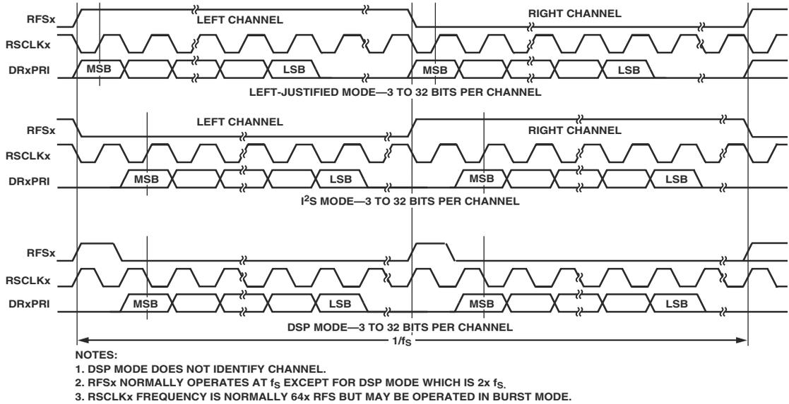
Figure 12-21. SPORT Stereo Serial Modes, Receive
