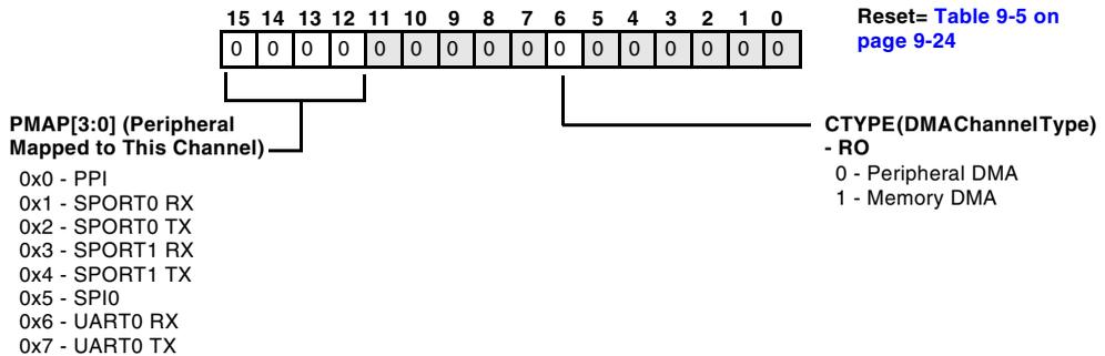
Figure 9-12. DMA Controller 0 Peripheral Map Register
