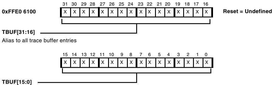
Figure 23-11. Trace Buffer Register
