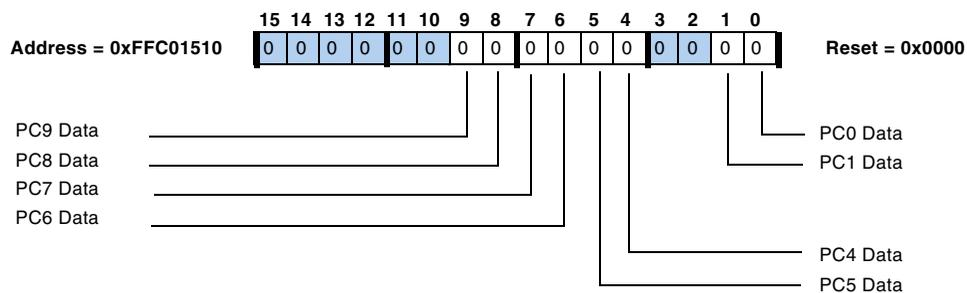
Figure 15-10. GPIO Port C Data Register
