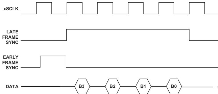
Figure 12-19. Normal Versus Alternate Framing
