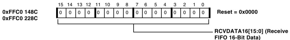
Figure 20-19. TWI FIFO Receive Data Double Byte Registers
