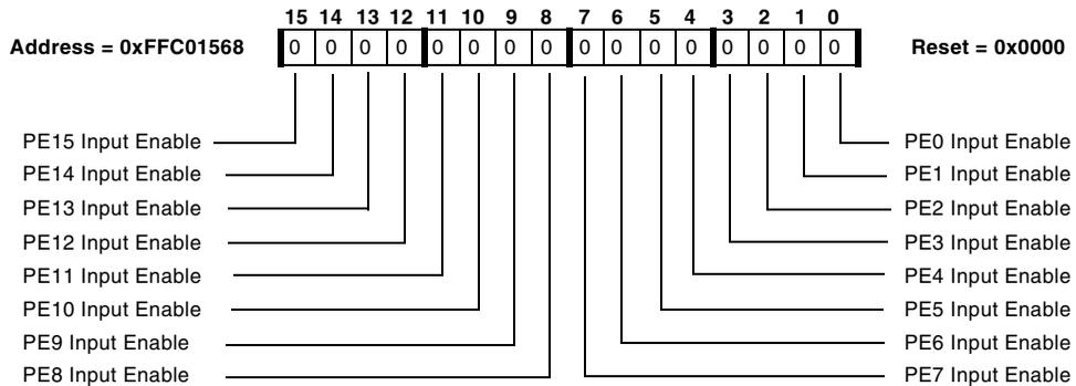
Figure 15-9. GPIO Port E Input Enable Register
