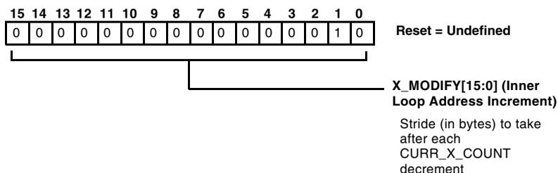
Figure 9-5. Inner Loop Address Increment Register
