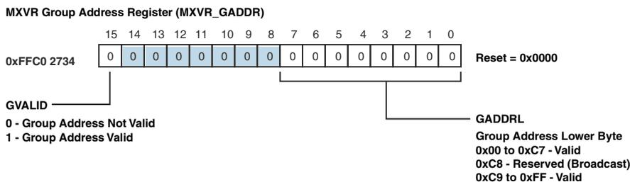
Figure 21-17. MXVR Group Address Register (MXVR\_GADDR)
