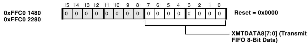
Figure 20-14. TWI FIFO Transmit Data Single Byte Registers
