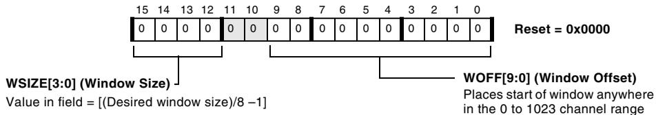
Figure 12-23. SPORTx Multichannel Configuration Register 1
