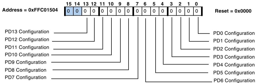
Figure 15-2. GPIO Port D Configuration Register
