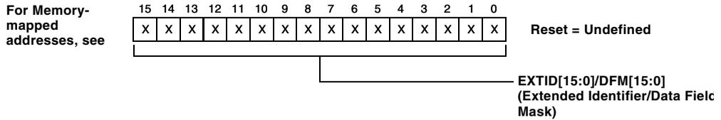
Figure 19-22. Acceptance Mask Register (L)
