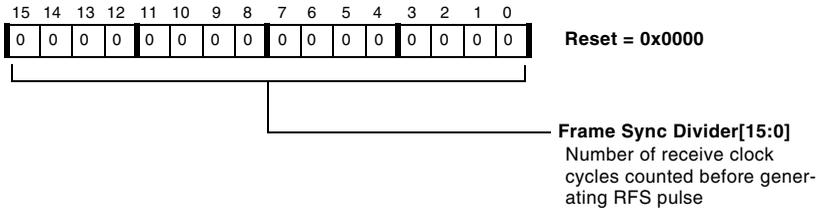
Figure 12-15. SPORTx Receive Frame Sync Divider Register
