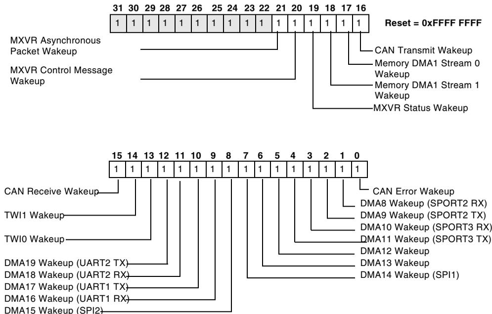
Figure 4-7. System Interrupt Wakeup-Enable Register 1 (SIC\_IWR1)
