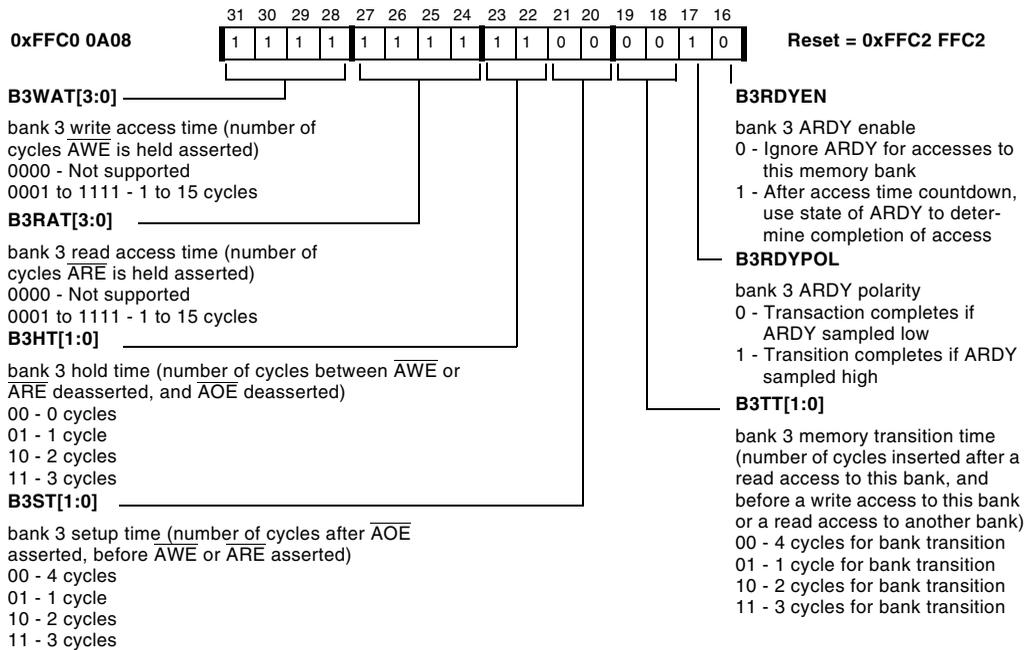
Figure 18-6. Asynchronous Memory Bank Control 1 Register (Bits 31–16)
