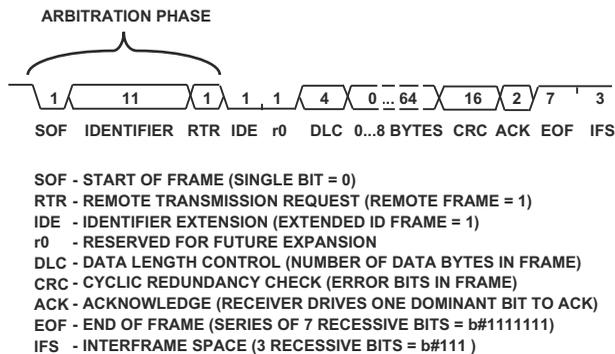
Figure 19-5. Standard CAN Frame
