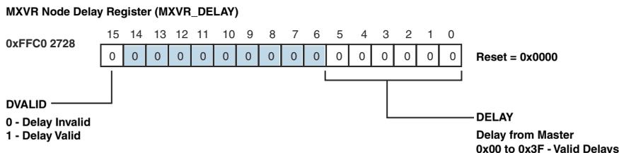
Figure 21-14. MXVR Node Frame Delay Register (MXVR\_DELAY)
