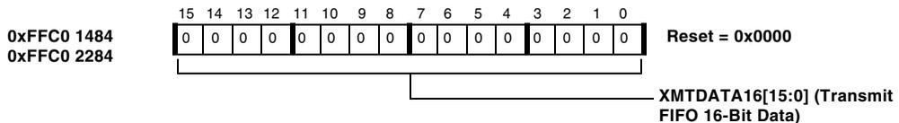
Figure 20-16. TWI FIFO Transmit Data Double Byte Registers
