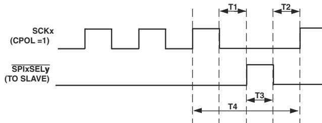
Figure 10-14. SPI Timing
