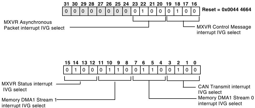
Figure 4-18. System Interrupt Assignment Register 6 (SIC\_IAR6)
