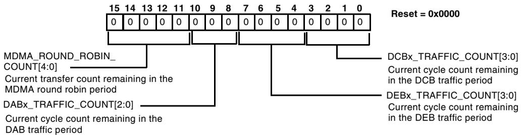
Figure 9-19. DMA Traffic Control Counter Register
