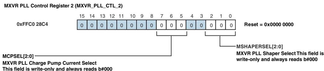
Figure 21-5. MXVR PLL Control Register 2 (MXVR\_PLL\_CTL\_2)
