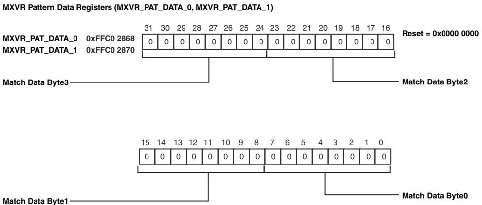
Figure 21-38. MXVR Pattern Data Registers (MXVR\_PAT\_DATA\_0, MXVR\_PAT\_DATA\_1)
