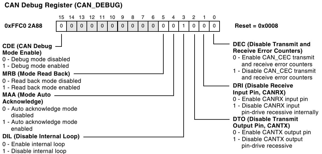
Figure 19-14. CAN Debug Register
