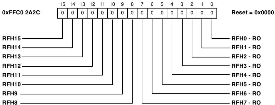
Figure 19-50. Remote Frame Handling Register 1
