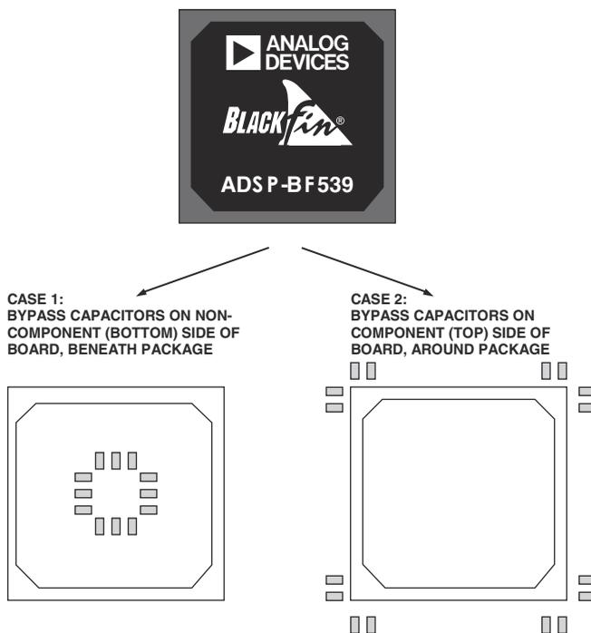
Figure 22-5. Bypass Capacitor Placement
