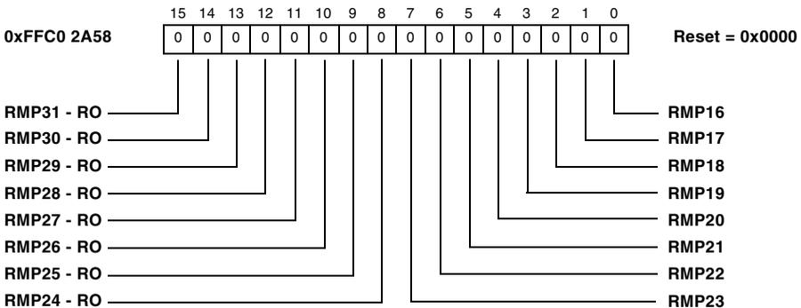
Figure 19-36. Receive Message Pending Register 2
