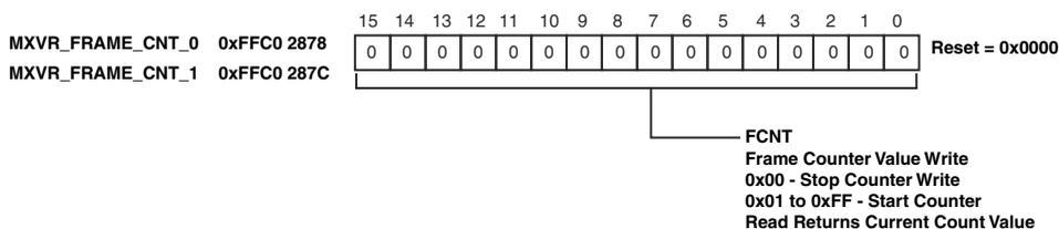
Figure 21-40. MXVR Frame Counter Registers (MXVR\_FRAME\_CNT\_0, MXVR\_FRAME\_CNT\_1)
