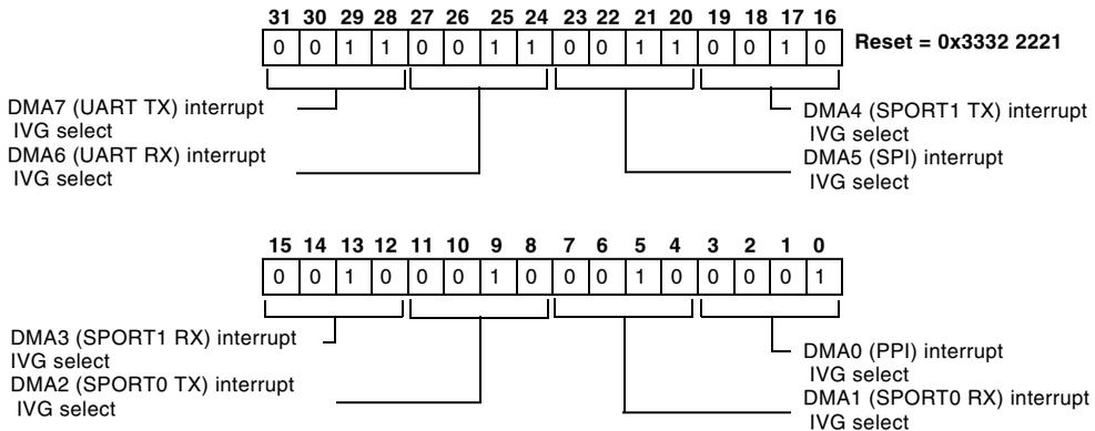
Figure 4-13. System Interrupt Assignment Register 1 (SIC\_IAR1)
