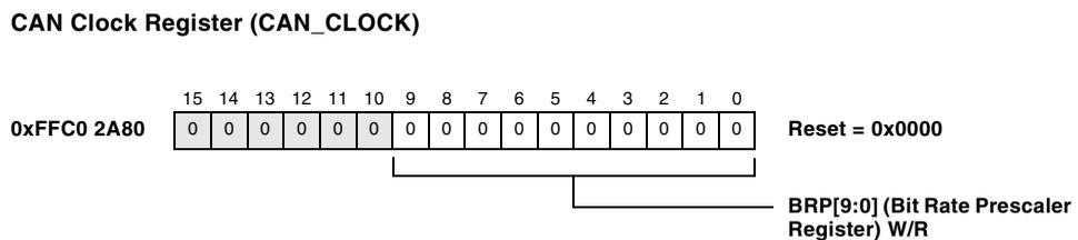
Figure 19-15. CAN Clock Register
