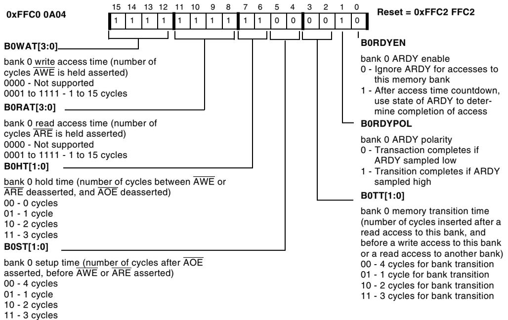
Figure 18-5. Asynchronous Memory Bank Control 0 Register (Bits 15–0)
