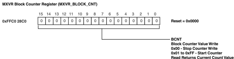
Figure 21-42. MXVR Block Counter Register (MXVR\_BLOCK\_CNT)
