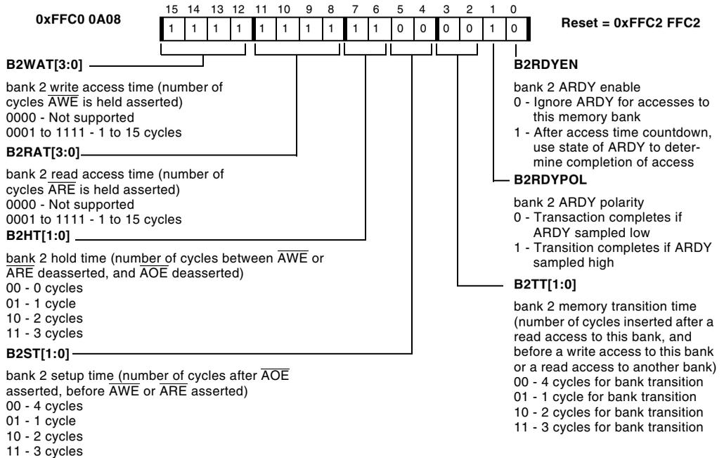
Figure 18-7. Asynchronous Memory Bank Control 1 Register (Bits 15–0)
