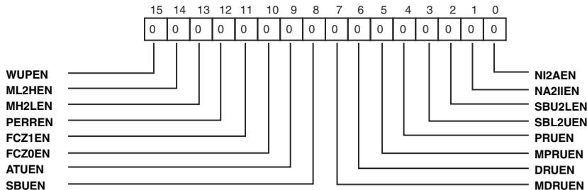
Figure 21-10. MXVR Interrupt Enable Register 0 (MXVR\_INT\_EN\_0)
