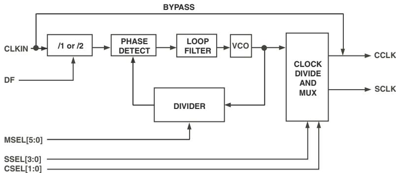
Figure 8-1. PLL Block Diagram
