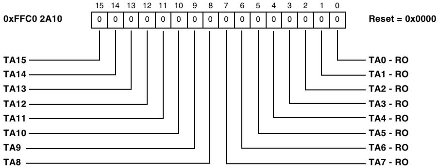
Figure 19-47. Transmission Acknowledge Register 1
