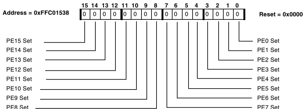
Figure 15-18. GPIO Port E Set Register
