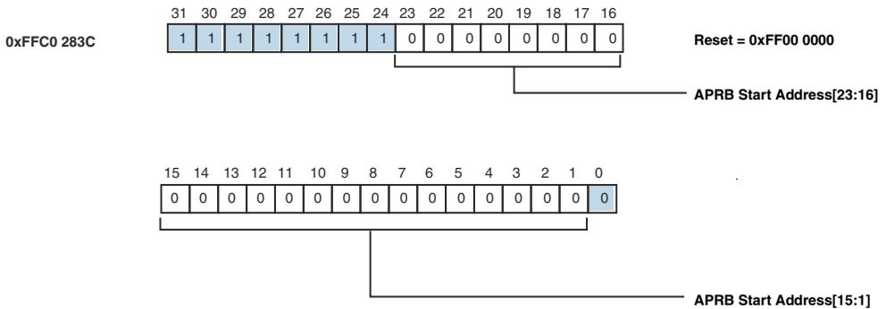
Figure 21-27. MXVR APRB Start Address Register (MXVR\_APRB\_START\_ADDR)
