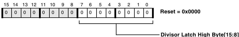
Figure 13-9. UART Divisor Latch Registers
