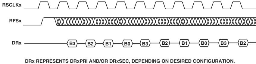
Figure 12-35. SPORT Receive, Unframed Mode, Alternate Framing
