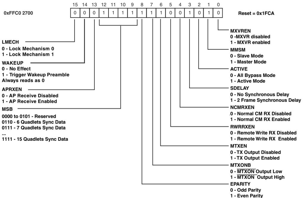
Figure 21-2. MXVR Configuration Register (MXVR\_CONFIG)
