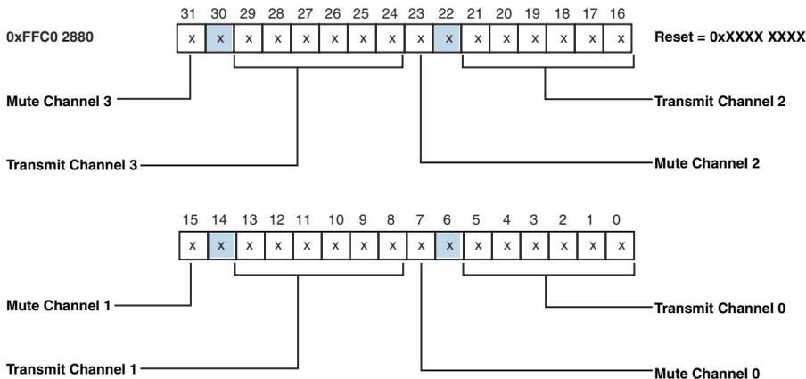
Figure 21-41. MXVR Routing Register 0 (MXVR\_ROUTING\_0)
