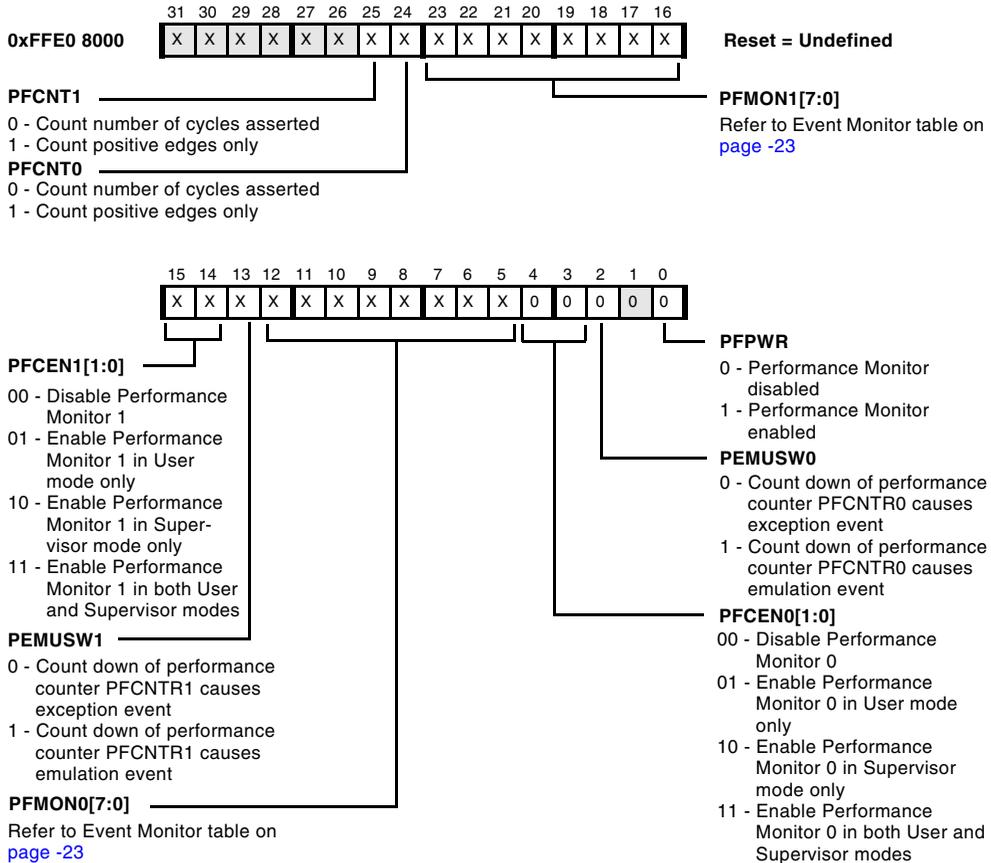
Figure 23-13. Performance Monitor Control Register
