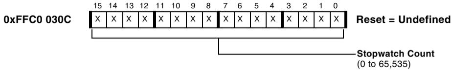
Figure 17-7. RTC Stopwatch Count Register
