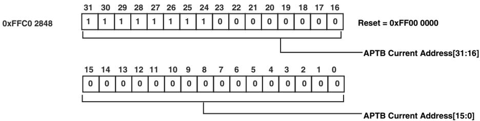
Figure 21-30. MXVR Asynchronous Packet Transmit Buffer Current Address Register (MXVR\_APTB\_CURR\_ADDR)
