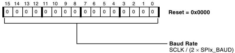
Figure 10-3. SPI Baud Rate Registers
