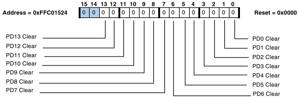
Figure 15-14. GPIO Port D Clear Register
