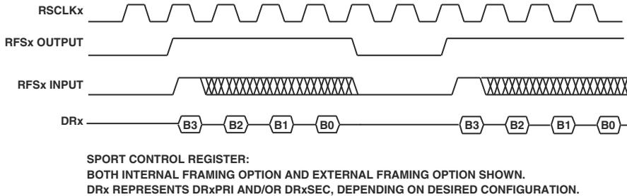
Figure 12-32. SPORT Receive, Alternate Framing
