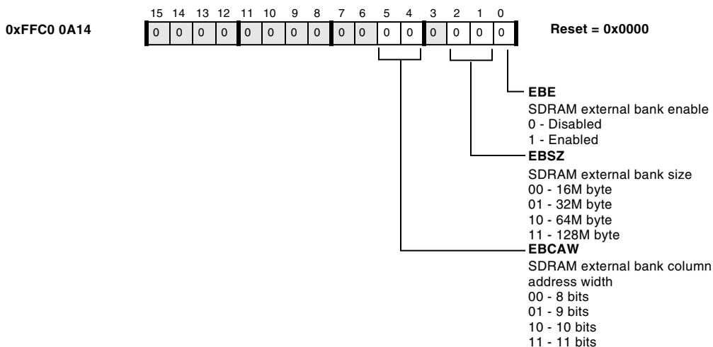
Figure 18-13. SDRAM Memory Bank Control Register
