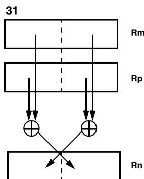
Figure 2-11. Cross Options for Dual 16-Bit ALU Operations
