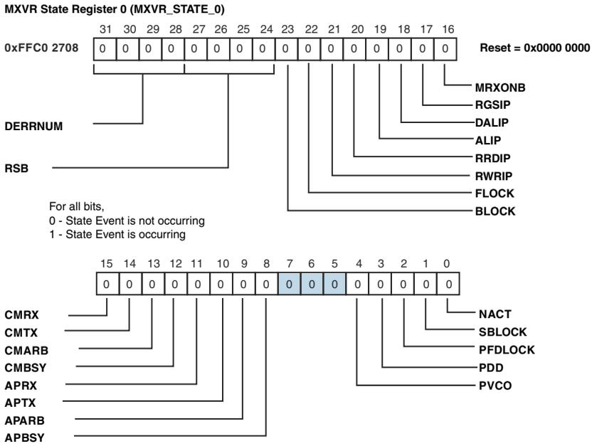
Figure 21-6. MXVR State Register (MXVR\_STATE\_0)
