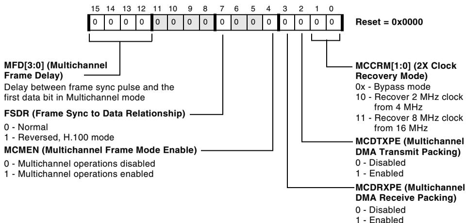
Figure 12-24. SPORTx Multichannel Configuration Register 2
