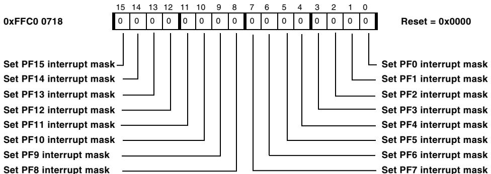
Figure 14-8. Flag Mask Interrupt A Set Register
