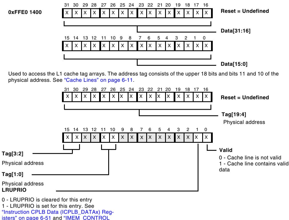
Figure 6-9. Instruction Test Data 0 Register
