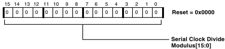
Figure 12-13. SPORTx Receive Serial Clock Divider Register
