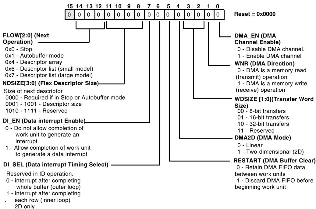
Figure 9-3. Configuration Register
