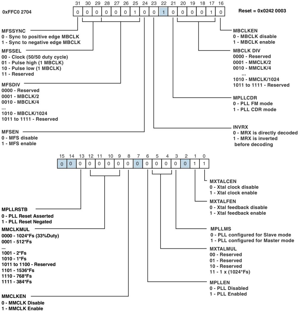
Figure 21-3. MXVR PLL Control Register 0 (MXVR\_PLL\_CTL\_0)
