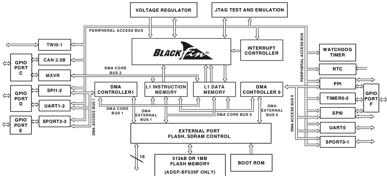
Figure 1-1. Processor Block Diagram
