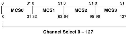
Figure 12-27. Multichannel Select Registers
