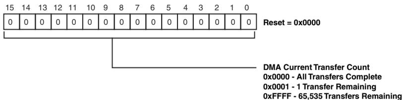
Figure 21-25. MXVR DMA Channel x Current Transfer Count Registers (MXVR\_DMAx\_CURR\_COUNT)
