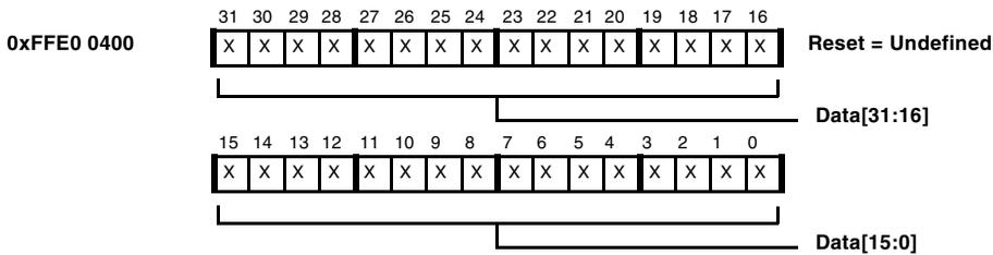
Used to access the L1 cache tag arrays. The address tag consists of the upper 18 bits and bit 11 of the physical address. See "Cache Lines" on page 6-11.
