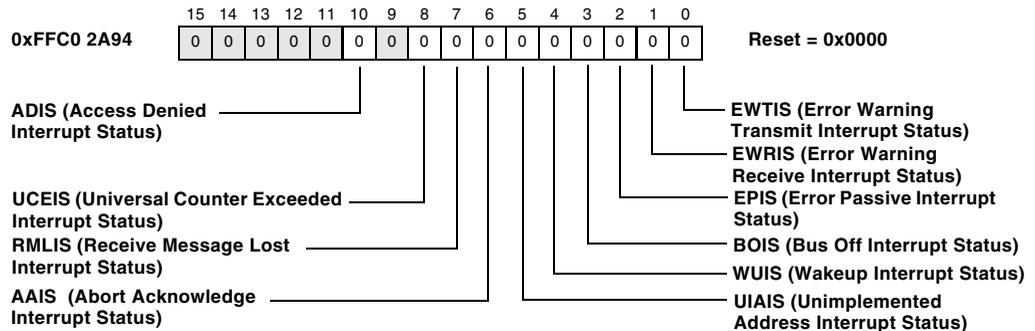
Figure 19-19. Global CAN Interrupt Status Register
