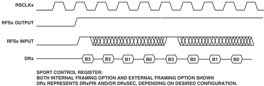
Figure 12-33. SPORT Continuous Receive, Alternate Framing
