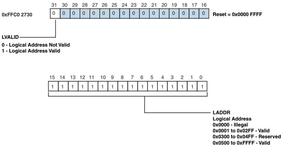
Figure 21-16. MXVR Logical Address Register (MXVR\_LADDR)
