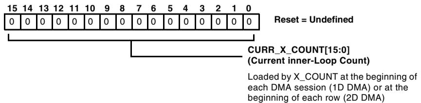
Figure 9-10. Current Inner Loop Count Register
