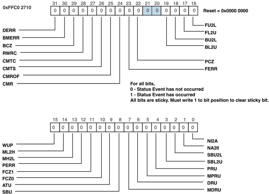
Figure 21-8. MXVR Interrupt Status Register 0 (MXVR\_INT\_STAT\_0)
