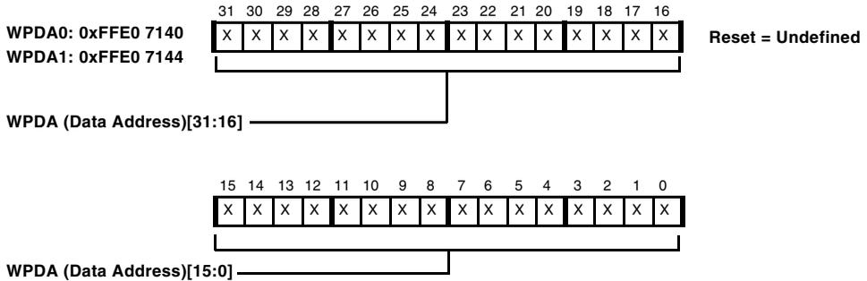
Figure 23-5. Data Watchpoint Address Registers
