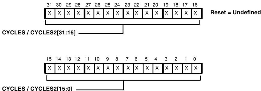
Figure 23-14. Execution Cycle Count Registers
