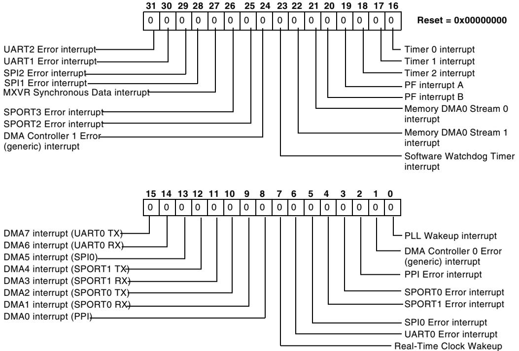
Figure 4-10. System Interrupt Mask Register 0 (SIC\_IMASK0)
