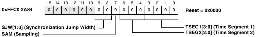
Figure 19-16. CAN Timing Register
