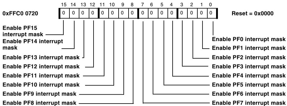
Figure 14-11. Flag Mask Interrupt B Data Register
