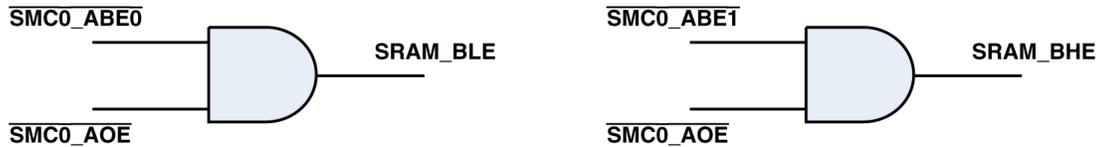
For SMC read operations, the  $\overline{\text{SMC0\_AOE}}$  signal is low. This drives the  $\overline{\text{SRAM\_BHE}}$  and  $\overline{\text{SRAM\_BLE}}$  signals low. This external logic does not affect the SMC write operations, as the  $\overline{\text{SMC0\_AOE}}$  signal is high during write operations.
