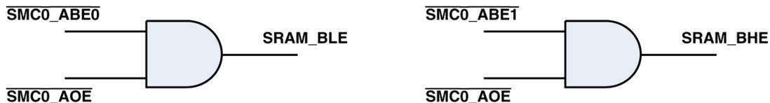
For SMC read operations, the SMC0\_AOE signal is low. This drives the SRAM\_BHE and SRAM\_BLE signals low. This external logic does not affect the SMC write operations, as the SMC0\_AOE signal is high during write operations.
