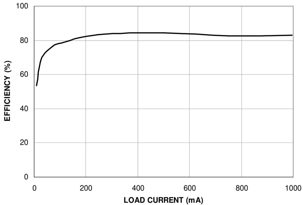
Figure 2. DC977 Typical Efficiency ( $T_A = 25^\circ\text{C}$ ,  $V_{OUT} = 3.3\text{V}$ )
