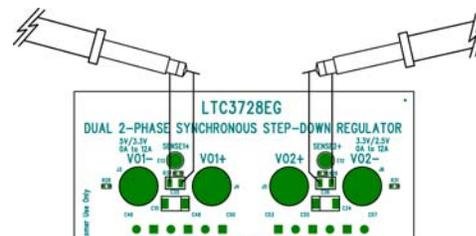
Figure 2. Output ripple measurement.
