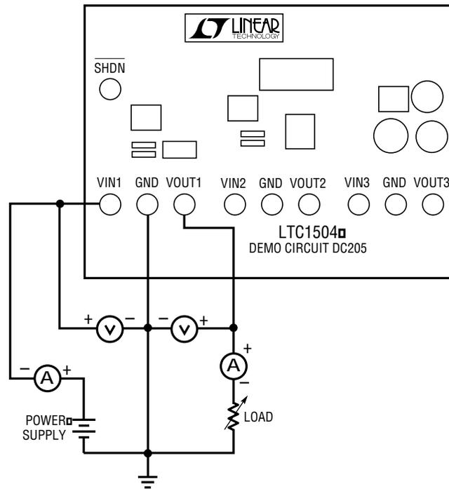
2. Turn on the input power supply and observe the output. The DC205 “high performance” circuit is programmed to generate 2.85V from a 5V input (for the “low profile” and “low cost” circuits, the output is set to 3.3V). The circuit will deliver up to 500mA at 2.85V (500mA at 3.3V for the “low profile” and “low cost” circuits).
