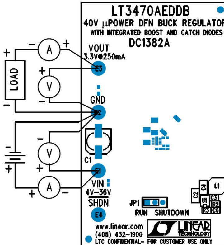
INSTALL SHUNT AT JP1 : PINS 1&2 = RUN
