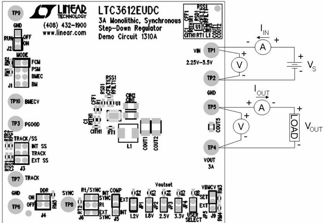
Figure 1. Proper Equipment Measurement Set-Up
