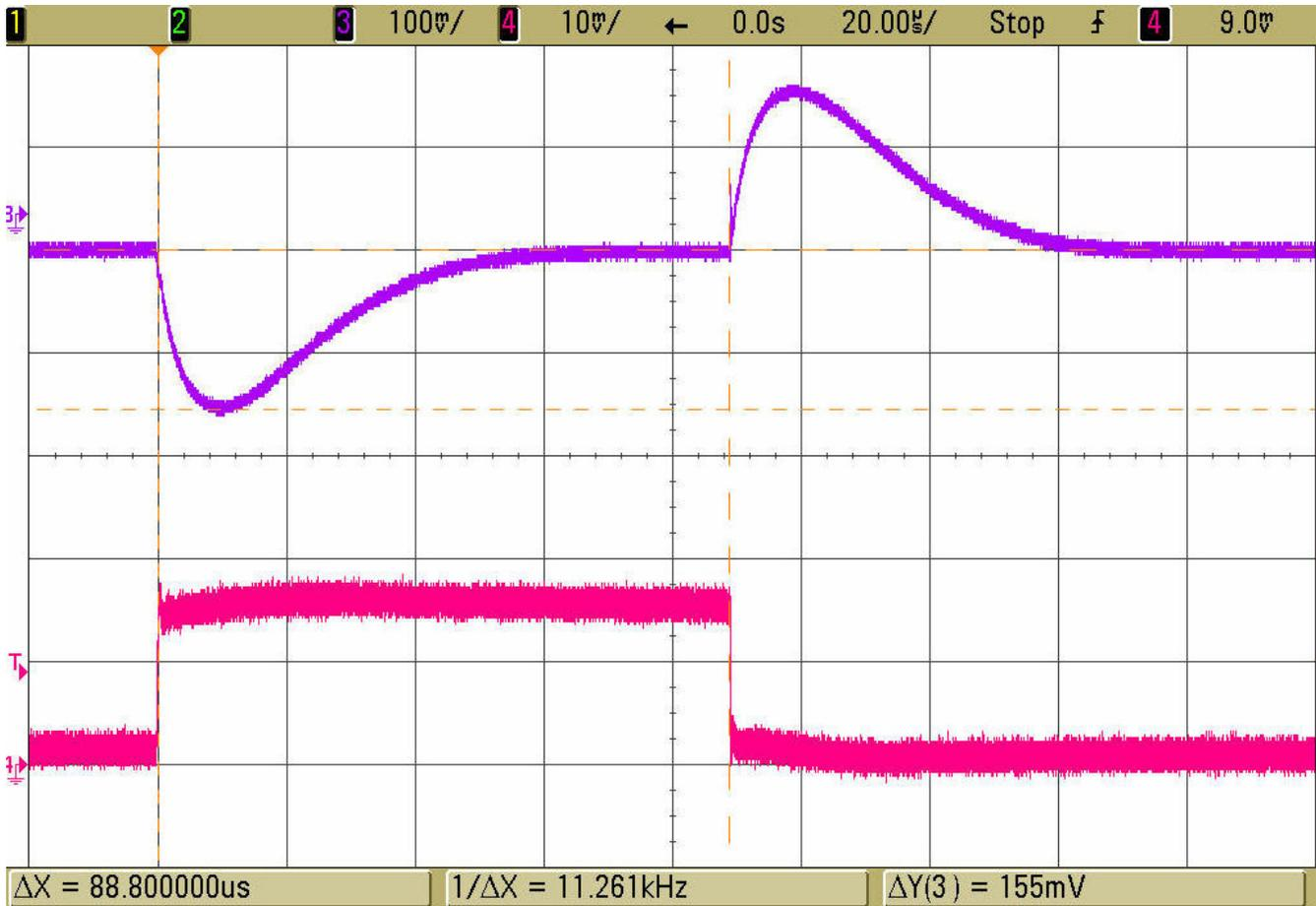
Figure 4. Load Step Response
