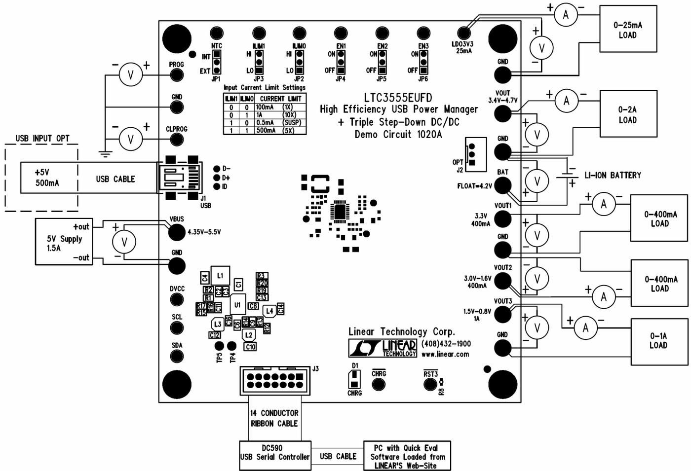
FIGURE 2: Proper Measurement Equipment Setup for DC1020
