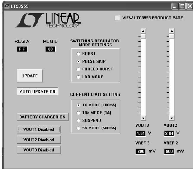
**FIGURE 1: Graphical User Interface Demonstration Software for DC1020.**
