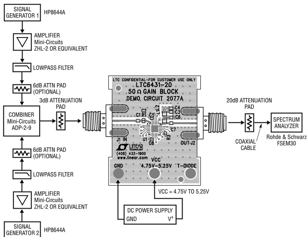
Figure 3. Proper Equipment Setup for IP3 Measurement
