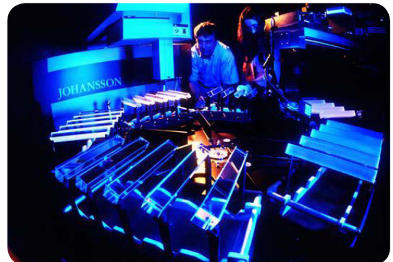
ADI's AD9042 ADCs measure the energy absorbed by these lead tungstate crystals (photograph courtesy of CERN).
