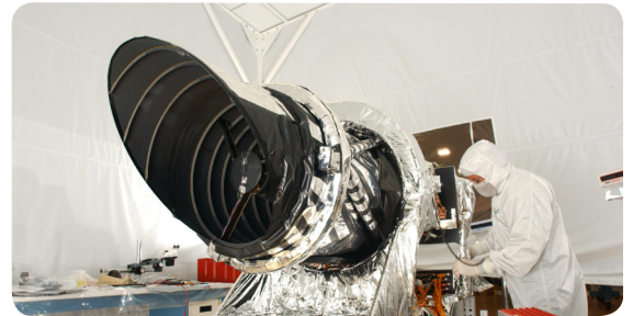
A worker at Ball Aerospace prepares the HiRISE camera for attachment to the Mars Reconnaissance Orbiter.
