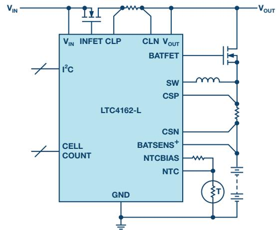
Figure 1. Typical application circuit for the LTC4162-L.
