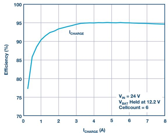
Figure 4. Lead acid charging efficiency with the LTC4015.
