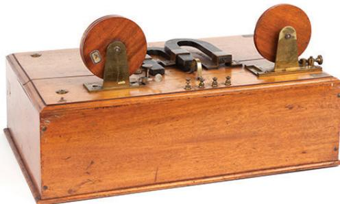
Figure 9. Magnetic detector as Marconi would have used.<sup>3</sup>
