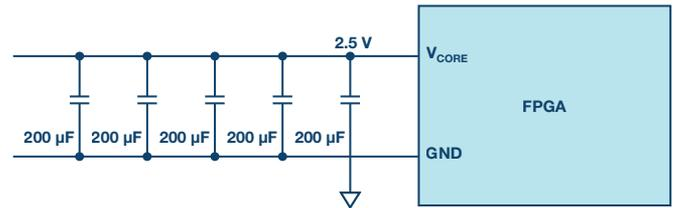
Figure 5. Input capacitor requirement of many FPGAs.
