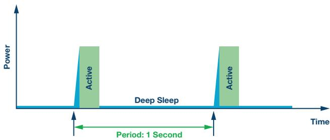
Figure 1. The ULPMark-CP has a period of 1 second. During this time, the device wakes up from deep-sleep mode, executes a fixed workload, and returns to deep-sleep mode.
