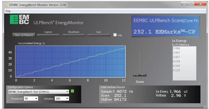
Figure 5. EnergyMonitor software—GUI.
