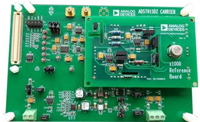
Figure 8. EVAL-AD5791SDZ with LTZ1000 reference board.
