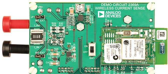
Figure 3. A complete wireless current sense circuit is implemented on a small PCB. The only physical connections are the banana jacks for the current to be measured. The wireless radio module is shown on the right. The circuit is powered from two AAA batteries connected on the back of the board.
