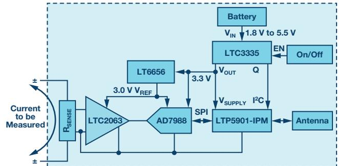
Figure 1. A low power, wireless current sense circuit is formed by a low power chopper op amp to amplify the sense voltage. It is digitized using a low power ADC and reference and connected to a SmartMesh IP wireless radio module. A low power, dc-to-dc converter conditions the battery and also keeps track of the charge drawn from the battery.
