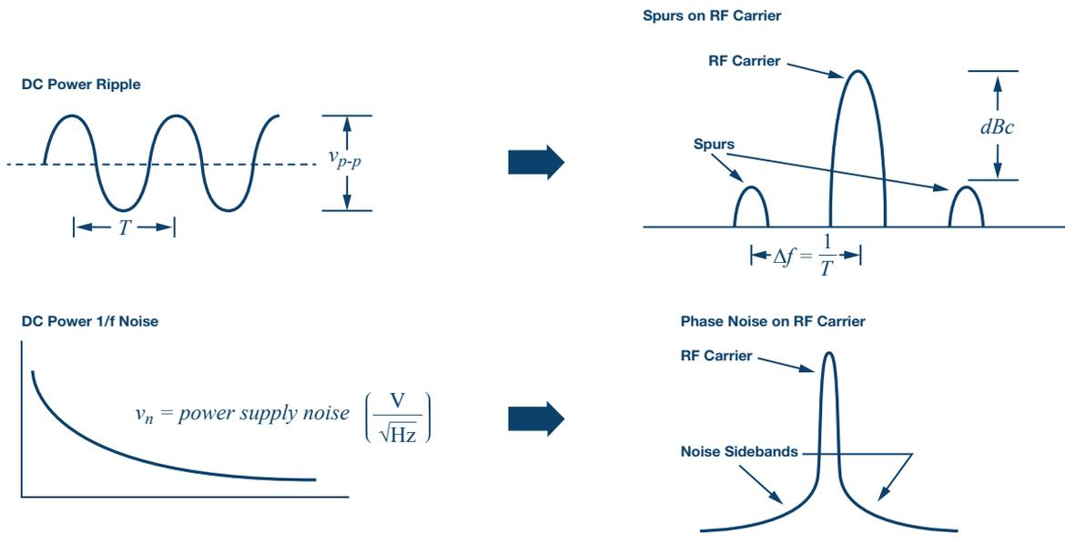
Figure 5. Power supply imperfections modulated on to the RF carrier.
