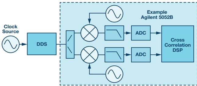
Figure 3. Absolute phase noise DDS test setup includes both DAC and oscillator noise.
