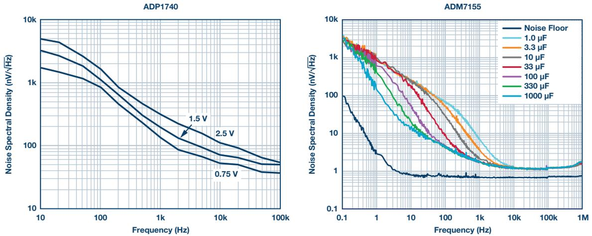
Figure 6. Regulator noise density comparison. Note the Y-axis units—the ADM7155 is an order of magnitude improved.
