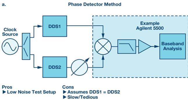
Figure 4a. DDS residual phase noise measurement using the phase detector method.
