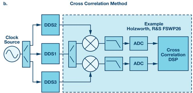
Figure 4b. DDS residual phase noise measurement using the cross correlation method.
