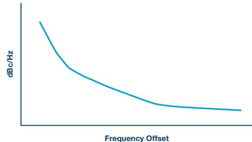
Figure 2. Phase noise plot method.
