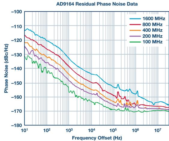
Figure 9. AD9164 residual phase noise measurements with low noise regulator improvement.
