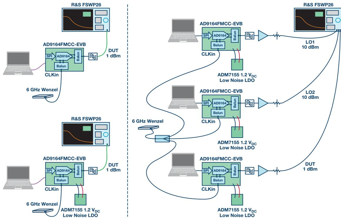
Figure 7. Test setups for AD9164 phase noise measurements.
