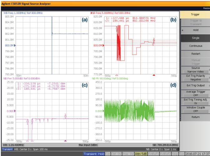
Figure 7. Hopping frequency from 804.5 MHz to 802 MHz with 500  $\mu$ s.
