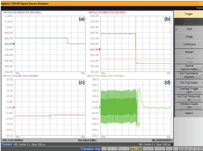
Figure 8. Hopping frequency from 882 MHz to 802 MHz within 20  $\mu$ s in fast lock mode.
