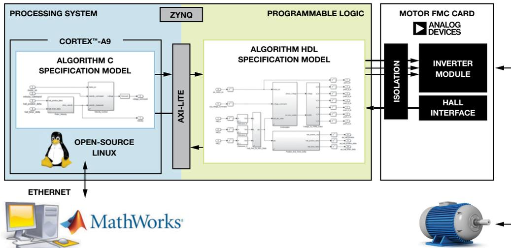
Figure 11. Controller implementation on the prototyping system.
