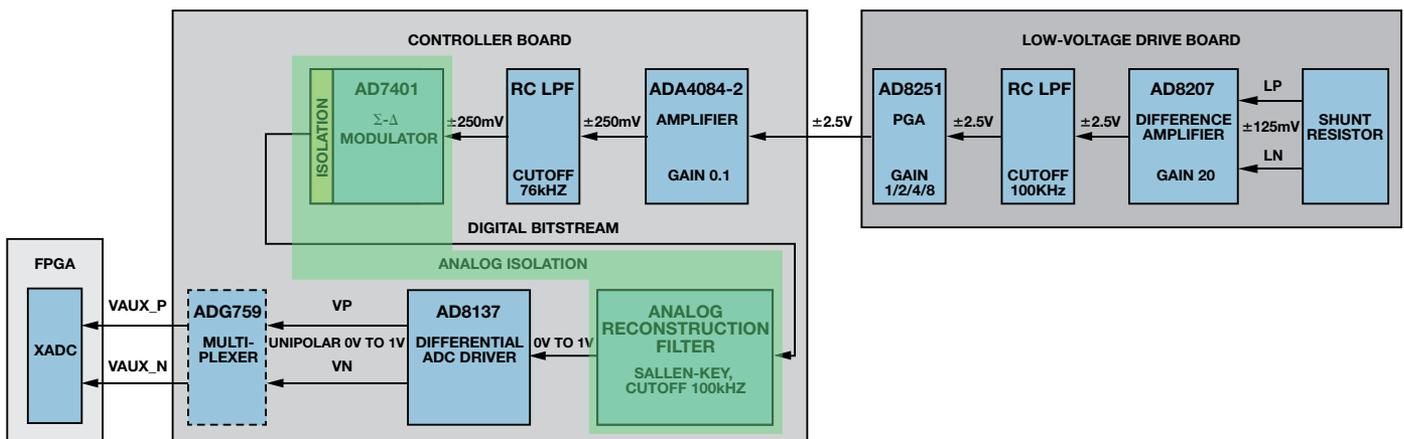
Figure 8. XADC signal measurement chain.
