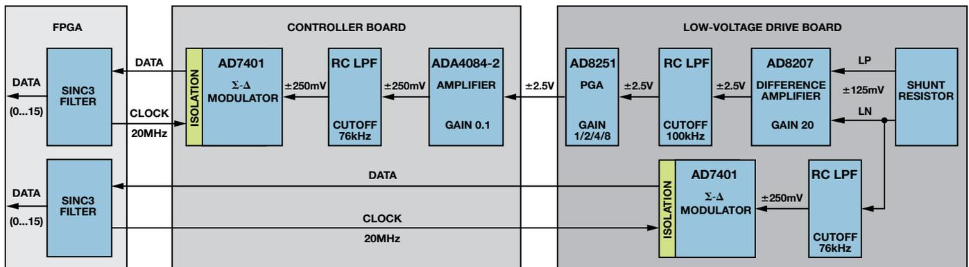
Figure 6. Phase-current signal chain.
