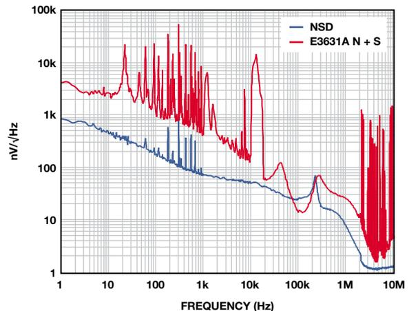
Figure 5. ADM7160 noise spectral density with 100 mV headroom.
