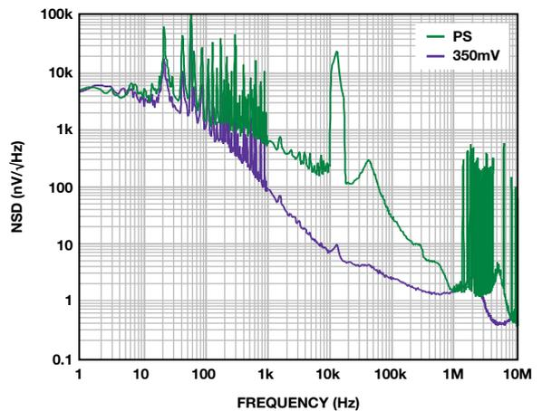
Figure 9. ADM7150 noise spectral density in dropout.
