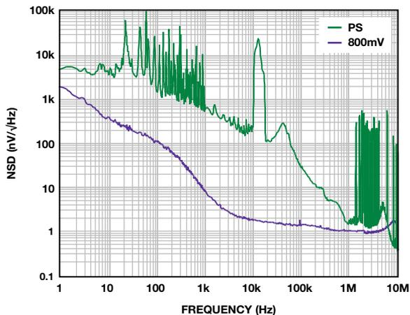
Figure 7. ADM7150 noise spectral density with 800-mV headroom.
