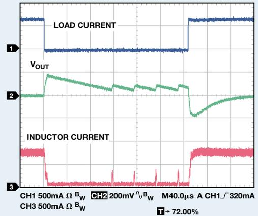
Figure E. ADP2370 load transient in power-saving mode.
