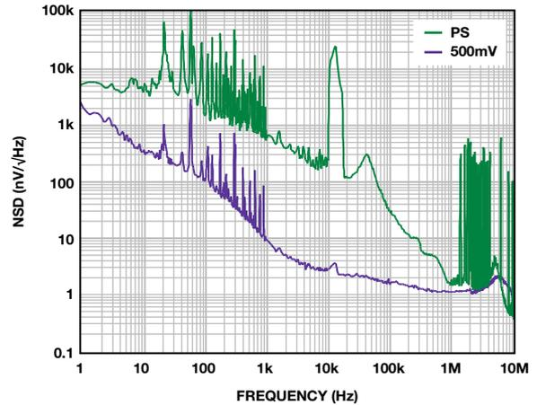
Figure 8. ADM7150 noise spectral density with 500-mV headroom.
