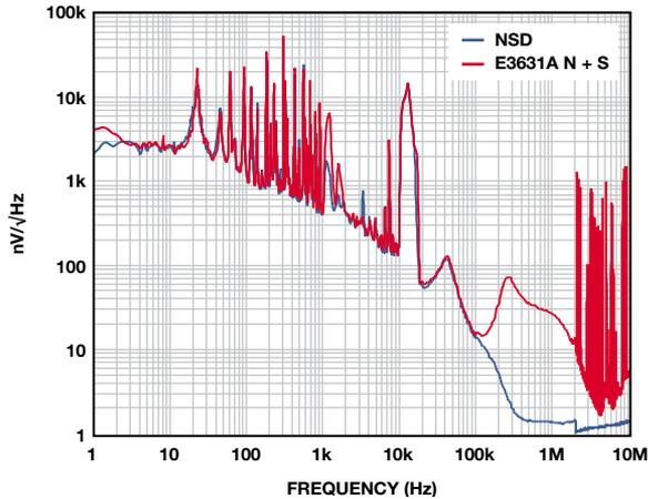
Figure 6. ADM7160 noise spectral density in dropout.
