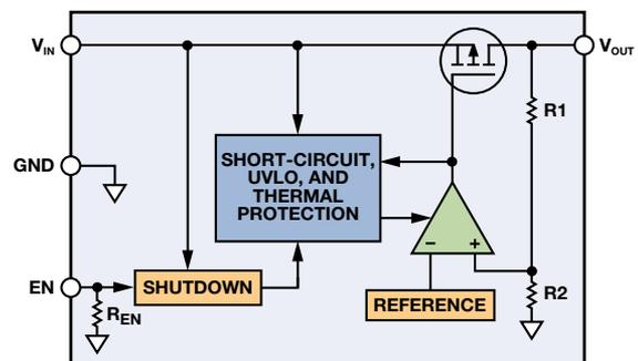
Figure 2. Block diagram of a low-dropout regulator.
