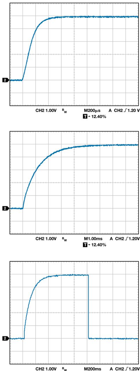
Figure 7. Start-up time of the ADP125 adjustable-output LDO (a) without noise-reduction network (b) with noise-reduction network,  $C_1 = 10$  nF, (c) with noise-reduction network,  $C_1 = 1$   $\mu$ F.
