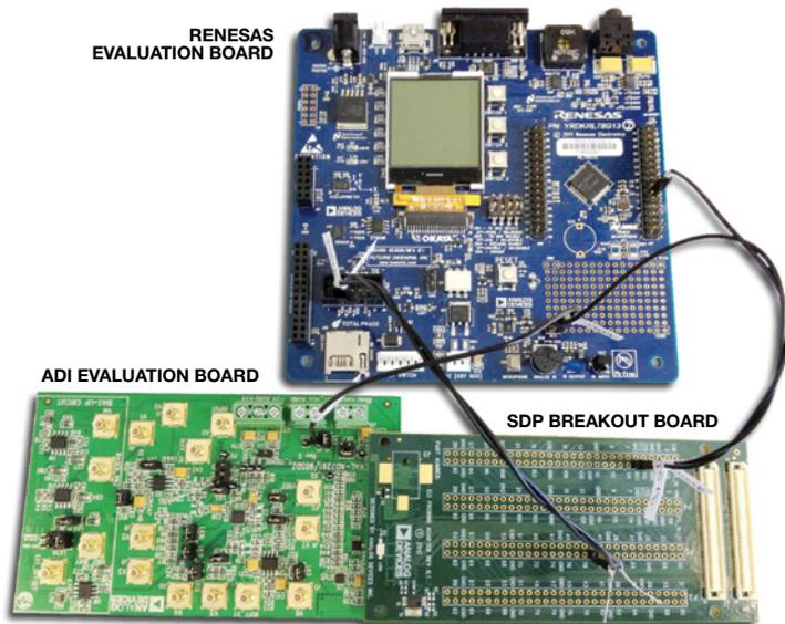
Figure 9. SDP breakout board connects the AD7291 evaluation board to Renesas evaluation board.
