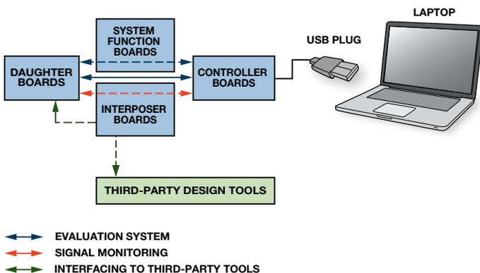
Figure 1. System demonstration platform overview.
