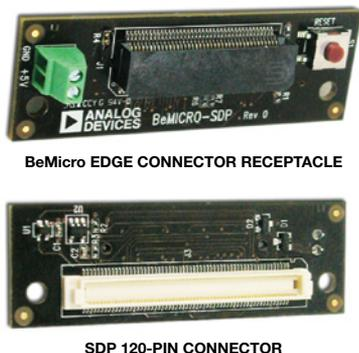
Figure 5. BeMicro SDK/SDP interposer.
