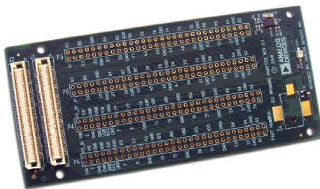
Figure 7. SDP breakout board.
