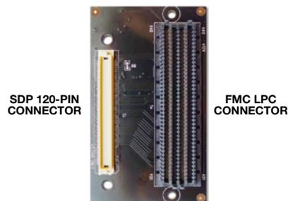
Figure 3. SDP-I-FMC interposer.
